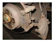
4. Unscrew hexagon 8 caliper mounting bolts to the hub, remove the caliper.
