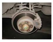
2. Old brake disc is usually due to wear a collar that prevents remove the caliper assembly with pads, so it's easier to remove the caliper frame by unscrewing the two screws.
