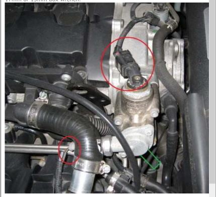
3) For clearance purposes, remove the hose fitting below the main PCV hose.
