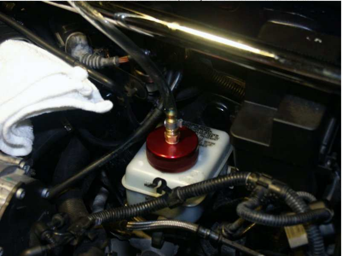
11. Now with an EMPTY Power Bleeder test the seal on the resevoir. This will save you the nightmare if their was an insufficient seal on the resevoir.
