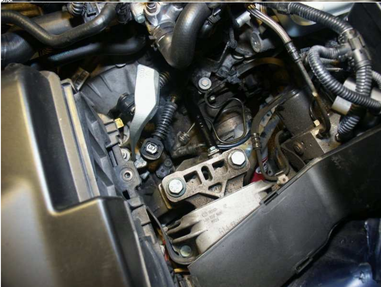
16. Close your bleed screw, and don't touch the clutch until the rest of the system is flushed. This will keep old fluid from potentially mixing with the new fluid.
