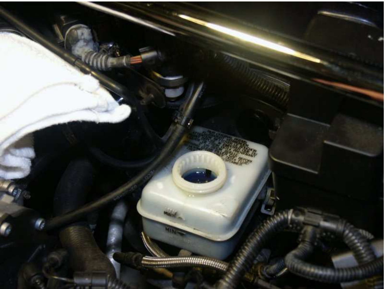
11. Now with an EMPTY Power Bleeder test the seal on the resevoir. This will save you the nightmare if their was an insufficient seal on the resevoir.
