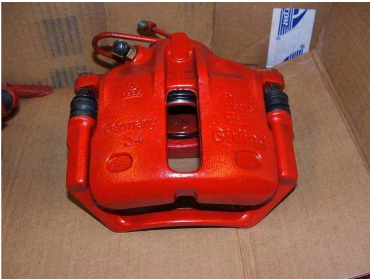
make sure the bleeder screw is facing up when installed to make sure you didnt install them upside down
