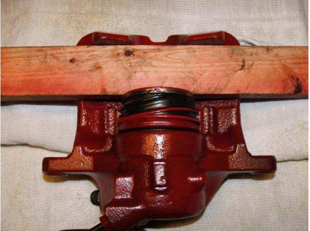
I was carefull with popping out the piston. 40psi worked for me. Use a bunch of brake clean in and out.
