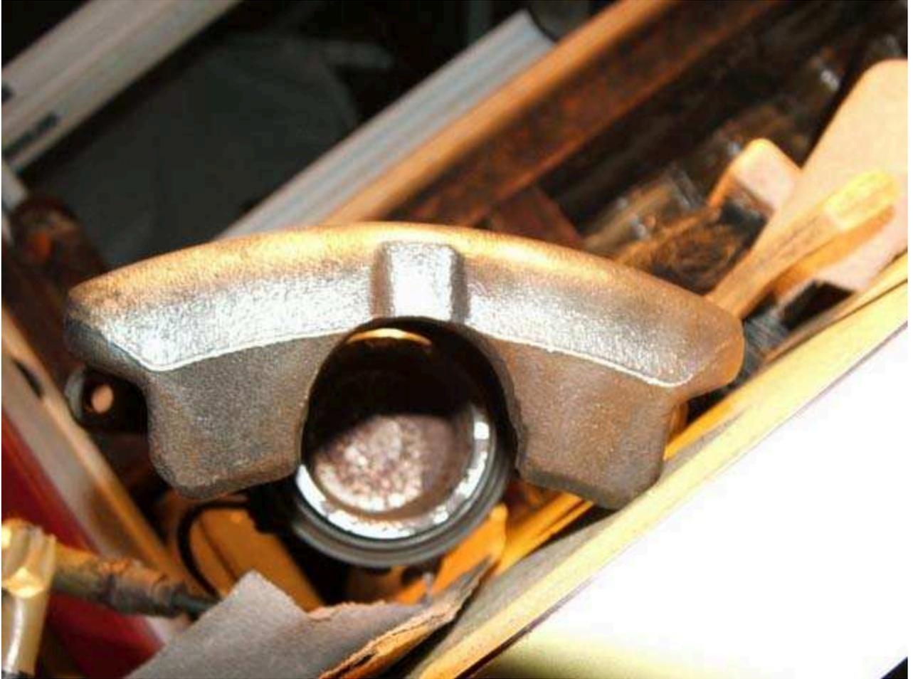
for all the fans file & smooth the casting marks on the carrier and calliper
