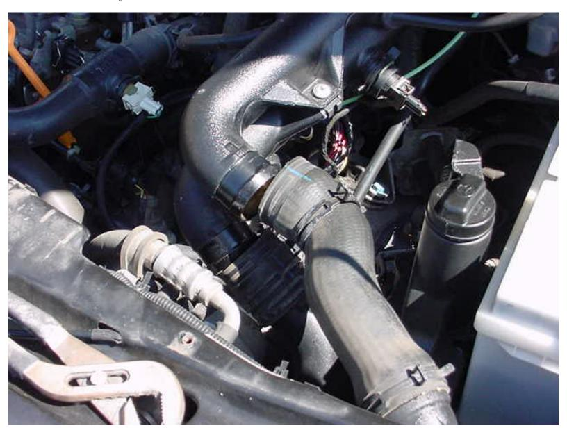
Viewing from the front of the car... Remove the rubber hoses from their mating plastic ones. Spring clamps are used here. Use some channel locks to open the spring clamps and slide them down the hoses. For future reference, we will be dumping all our liquids in the bottom hose.
