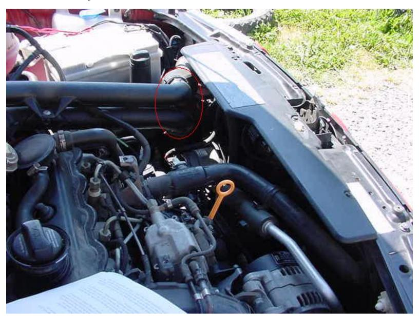
Here's a view of the area we will be working with on the top of the car. I also removed the plastic cover (still in place in this picture) directly behind the hood latch (8mm nuts holding this in place). The two circled hoses need to be disconnected.
