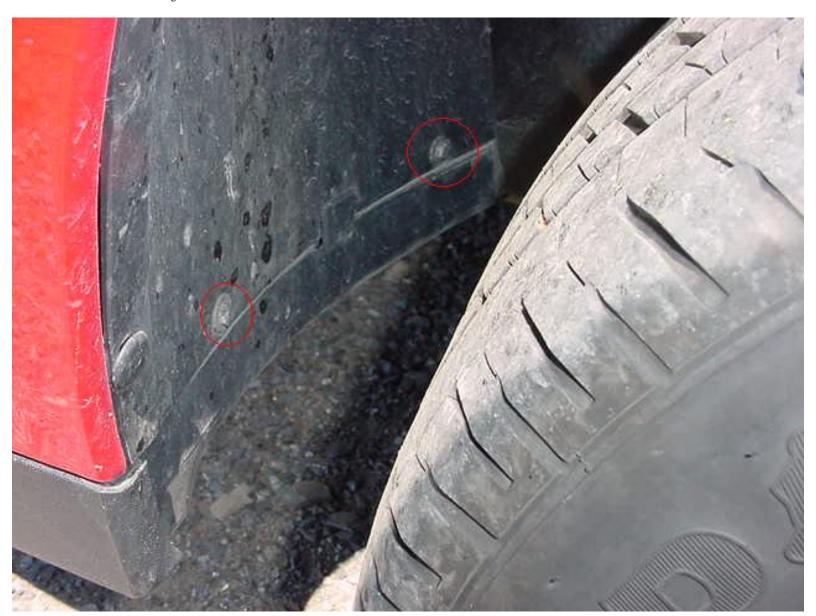
Now gain access to the bottom of the intercooler. I choose to jack up the driver's side of the car to make it easier. To remove the panel blocking access to the bottom of the intercooler, remove the two 7mm bolts on the inside of the wheel well (shown here) and also two Philips head screws under the car and along the front plastic valance.
