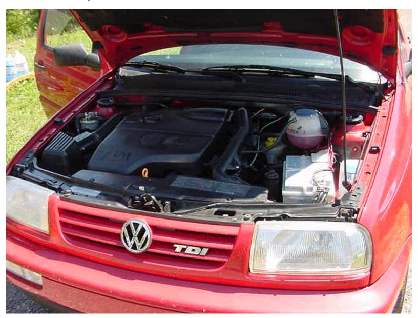
First things first - pop the hood. To make things easier for me, I elected to remove the engine cover (three 10mm bolts).
