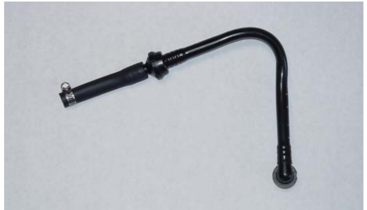
26. Remove section of brake booster hose between manifold port and check valve. This may require cutting the hose as shown to remove. Connect one end of supplied \frac{3}{8} " X 12" brake booster vacuum hose to check valve and the other end to the 90-degree hose barb located on rear of Supercharger housing. Use supplied \frac{1}{2} " hose clamp to secure hose.
