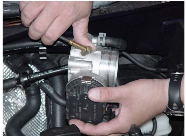
19. THROTTLE BODY INSTALLATION: Using the M6X100 (black) bolt supplied, insert into hose barb and rotate the 90-degree vacuum port fitting approximately 45-degrees as shown. Install throttle body with supplied gasket using factory bolts. Torque bolts to 7ft. lbs. Reconnect electrical connector to throttle position sensor.
