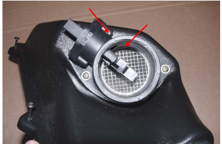
22. MAF AND AIR BOX COVER INSTALLATION: Remove O-ring from factory air box cover, lubricate, and transfer to new air box cover. Install MAF on new air box cover using factory screws. Now install air box cover to lower half using factory screws from stock cover. Snap on air pump hose, and re-install throttle body to air filter air intake hose. NOTE: If you do not have an air pump, you should have been provided a plain air box cover without a hole or fitting.
