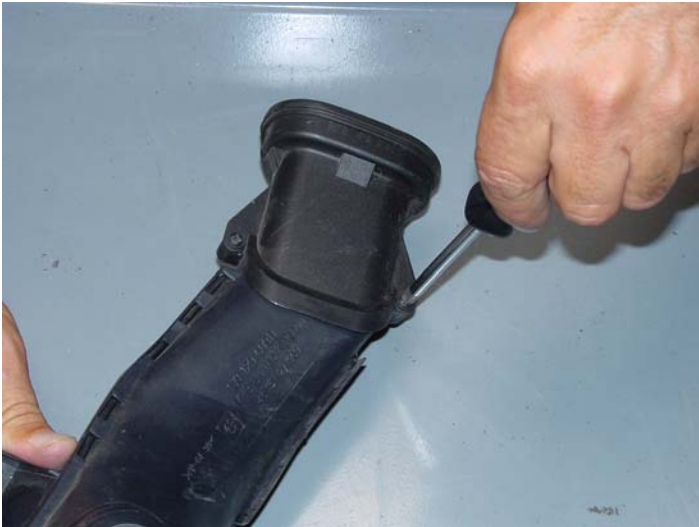
21D. Disassemble air duct by removing two (2) Phillips screws.
