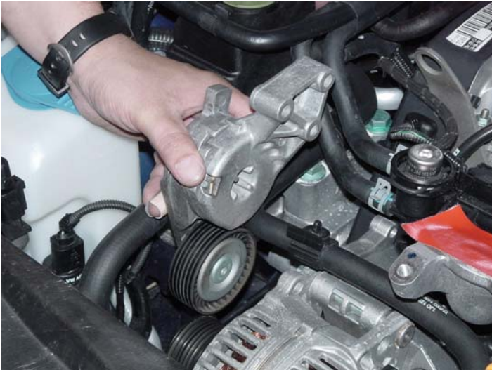
10. BELT TENSIONER REMOVAL: Using a 15mm open-end wrench, rotate tensioner to release tension on belt and remove the ribbed V-belt. Remove the three 13mm tensioner mounting bolts and remove tensioner assembly.
