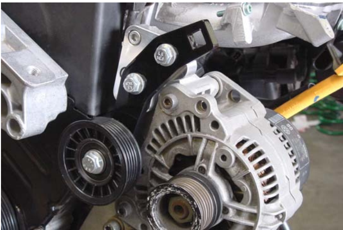
17. BELT TENSIONER ARM, PULLEY AND BELT INSTALLATION: Pulley has been pre-installed on arm. Install tensioner arm with pulley, and tighten supplied 13mm bolts hand tight. Install new supplied belt according to Belt Path diagram. Double check to be sure that the belt is properly seated into ALL the grooves on each pulley.
