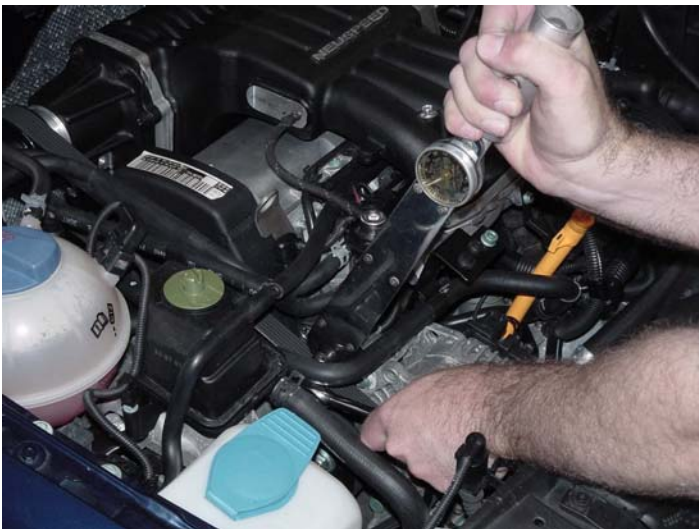
18. BELT TENSIONING: Using a 1/2" drive torque wrench, tension belt to 35ft. lbs. Now tighten tensioner arm bolts to 18ft. lbs.
