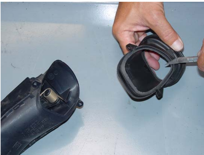
21E. Locate mesh screen and cut around perimeter of air duct to remove. (Mesh screen has already been removed from picture).
