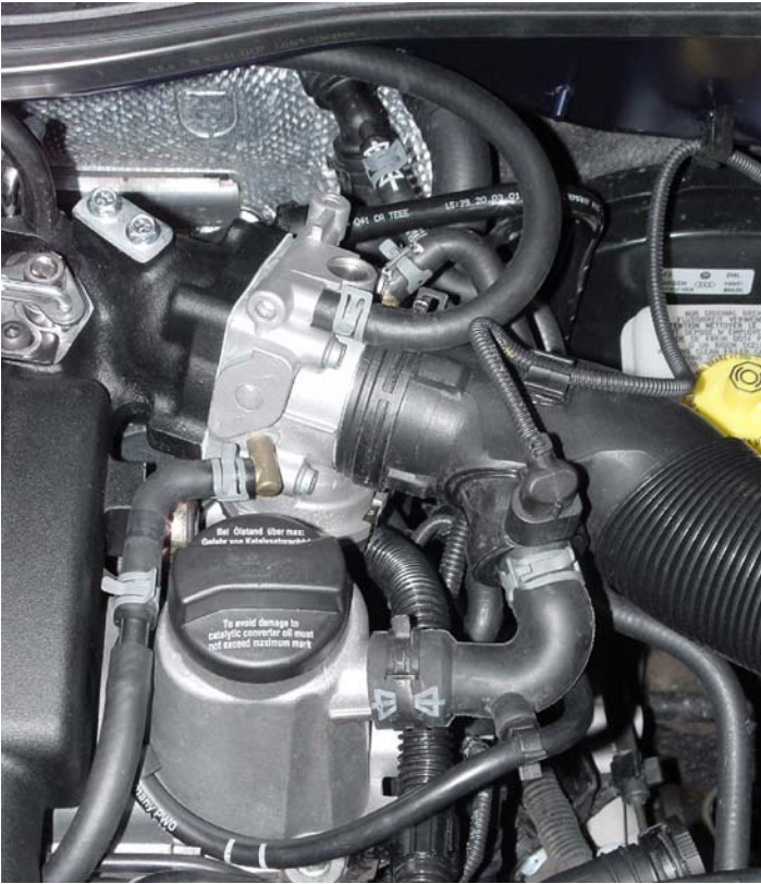
24. Using factory clamps, install supplied PCV hose as shown.
