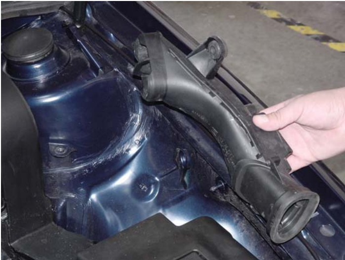
21C. Remove air duct by removing M6 nut (10mm hex) and sliding duct up and out towards windshield.
