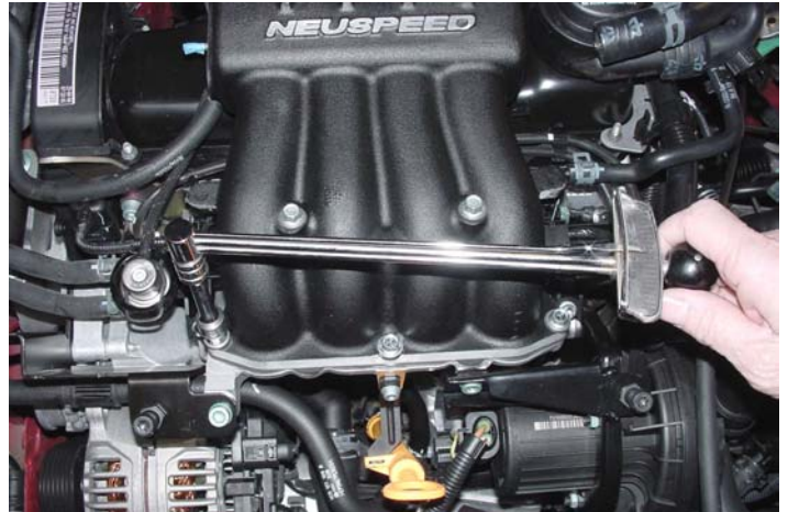
12. SUPERCHARGER INSTALLATION: First assemble the supplied new stainless steel/neoprene backed washers on the supplied new (3) M6X25mm and (2)M6X95mm intake manifold bolts. Ensure that the steel side of the washers are in contact with the heads of the bolts, and apply a small amount of NEUSPEED special grease to the neoprene side. With the Supercharger on the bench, and the mounting flange vertical, position the intake manifold gasket on the inlet runner flange and align ports. Be very careful here because the gasket only fits one-way – double check alignment of ports and bolt mounting holes! Insert bolts into proper holes to hold gasket in place. Remove tape covering lower intake ports, and lower Supercharger onto lower intake runners. Carefully support backside of Supercharger until you have run mounting bolts down and torqued to 44inch lbs. (3.6 ft. lbs.). Now you must check to see if the Driver Side Rear Support Bracket is in alignment with threaded hole on Supercharger. Bolt MUST align perfectly with hole . If not, determine amount of adjustment (up-or-down) to properly position rod end. You will need to remove Supercharger – make adjustment, re-torque bolts and try again. NOTE: Supercharger MUST be torqued to proper setting BEFORE checking/installing bolt! When you have a perfect fit, apply Loctite and torque Supercharger Rear Support bolt M8X35mm to 15ft. lbs, and tighten jam nut on rod end if you made an adjustment. NOTE: This step is very important – you MUST take time to do it right!
