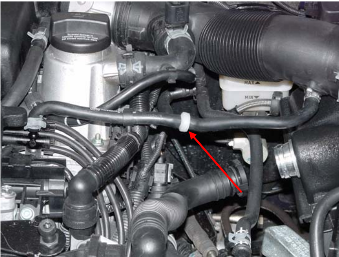
25. CHECK VALVE INSTALLATION: Cut fuel injector vacuum line halfway between fuel rail and air intake hose – insert new check valve supplied. Check valve MUST be installed with conical end (red dot) facing engine!
