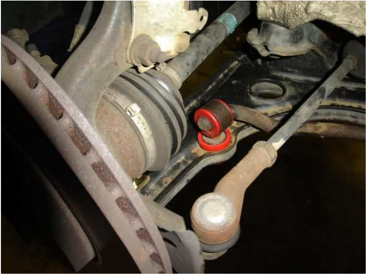
(Sway bar bushings installed)
