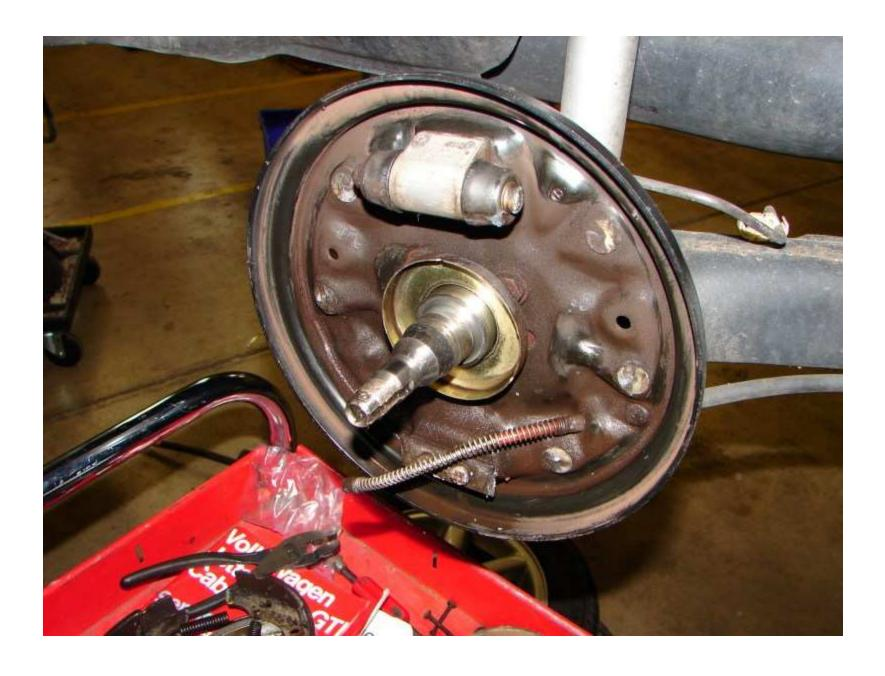
**Note**: We have yet to play with the wheel cylinder at this point. IF fluid starts to come out of the wheel cylinder its ok. Again, make sure the cap is on the master cylinder, if not a LOT more fluid will come out. If the master cylinder "goes dry" you have a bigger issue on your hands. So every once and a while keep an eye out for low fluid or leaks.
