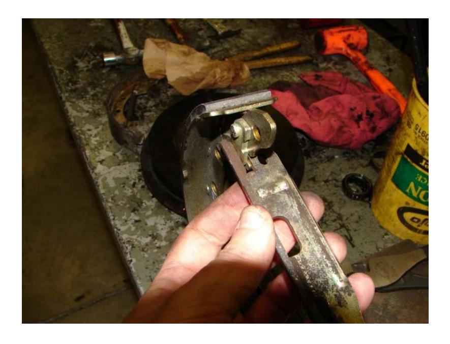
This is a close-up of the brake shoe and pushrod with the springs off of it. This is a handy picture since you CAN install things wrong at this point.
