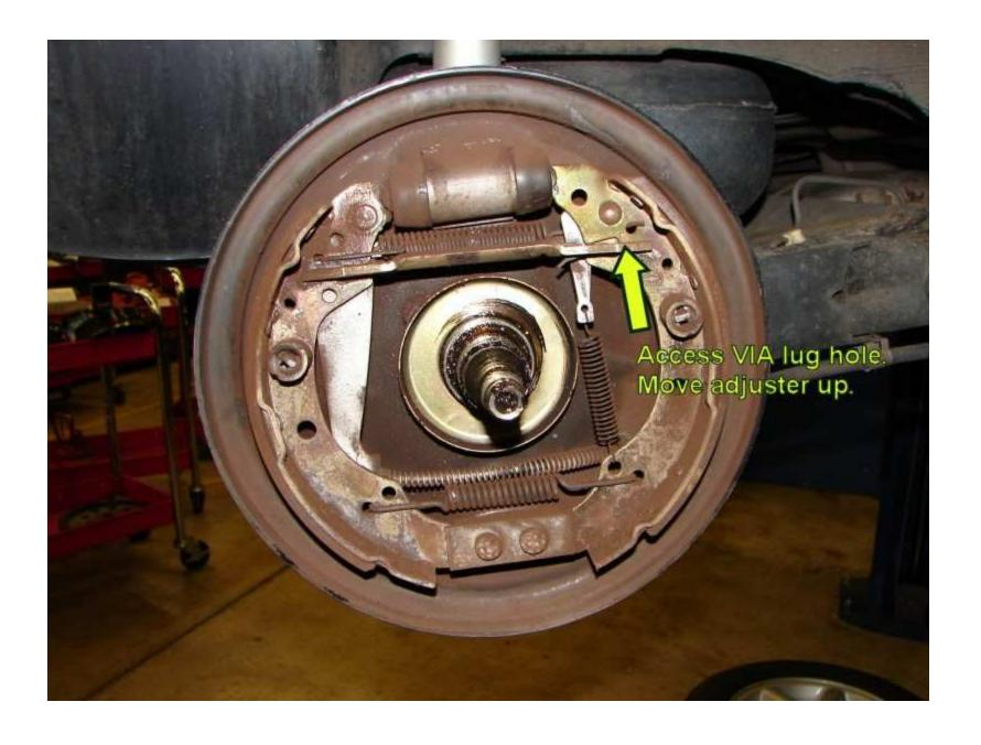
If the rear drum cannot come off the spindle as you pull it towards yourself (once the cotter pin, cage, spindle nut and outer bearing are off) chances are the shoes are worn and have left a ridge on the backside of the drum. You'll need to retract the adjuster. Do this by spinning the drum so you can insert a flathead screwdriver into one of the lug holes. From there flick up the retractor and the shoes should retract and then you should be able to take off the drum.
