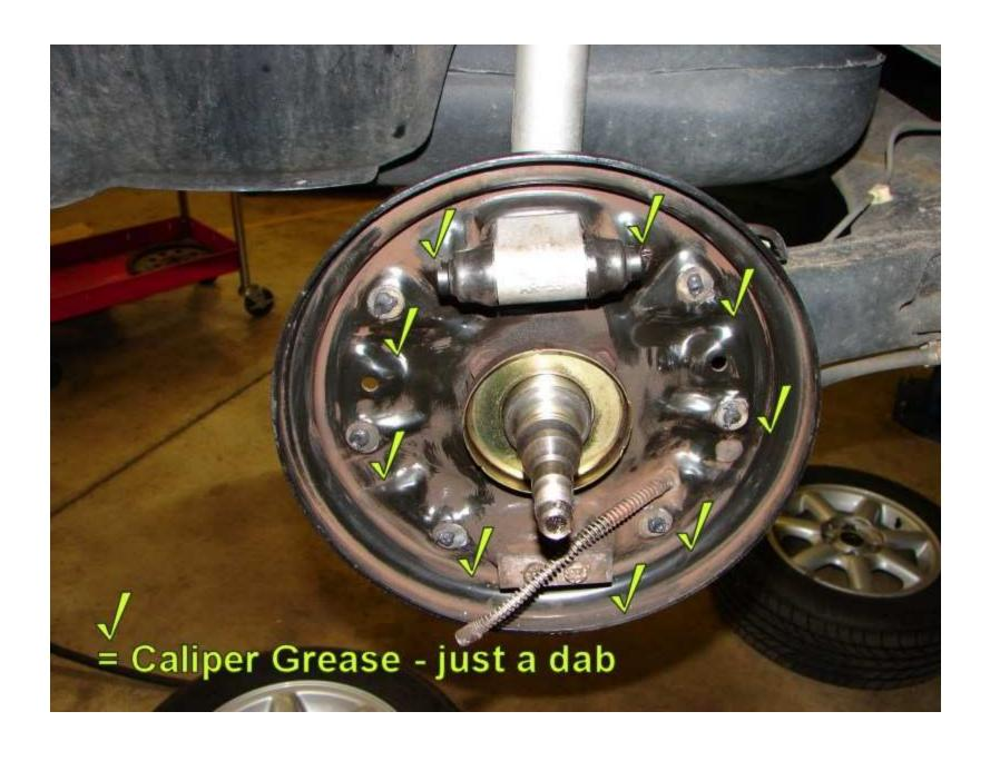
Lube the backing plate "buttons" with a small dab of caliper lube. Dab grease at the anchors and ears of the wheel cylinders. This step is important in order to prevent noise and binding.
