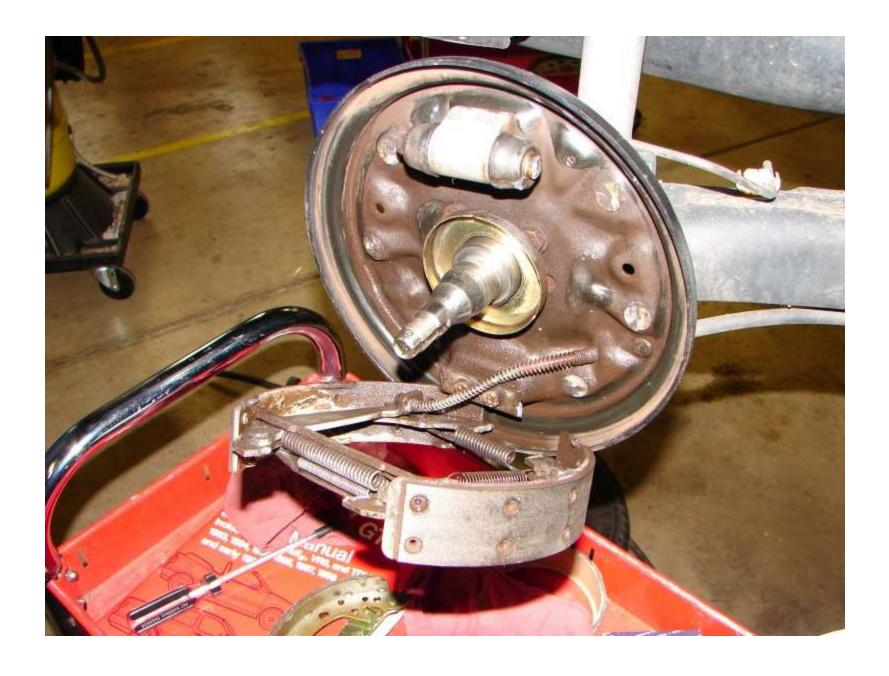
And the parking brake cable is the part left holding it to the car.
