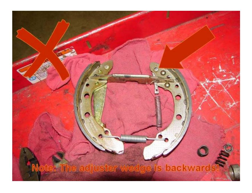
Here is my first try at putting the shoes back together. I installed the adjuster wedge backwards. If I left it like this, The brakes would work, but never self adjust.
