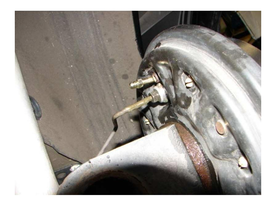
Allow the fluid to dribble out for a few seconds, again, for about a total time of two minuets. Keep an eye on the fluid level and refill it if it starts to drop below or to the low mark. Fill it slowly.
