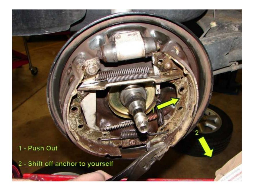
**Step 9** - Carefully shift off the brake drum shoes and springs and have them lie flat. This will require you to shim the wheel cylinder pistons some. Don't worry they are supposed to move. Just don't push them too far. Again leave the springs ALL on the shoes. They help create a "frame" that will aid you in taking things apart.
