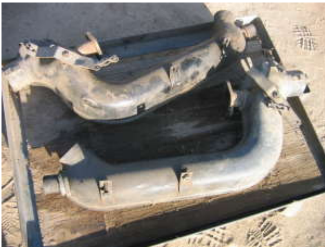
Fig 4 - Set of Heater Boxes removed from vehicle
