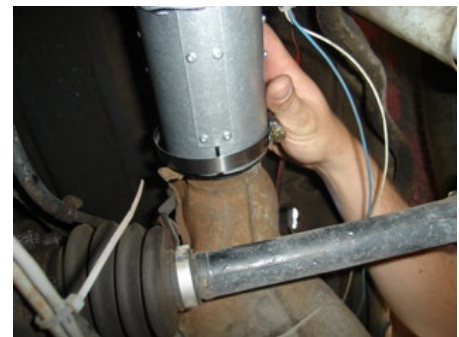
Fig 7b - Installing blower assm onto heater box
