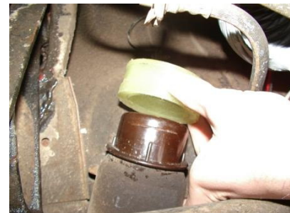
Fig 8 - Slide bushing onto plastic fitting on the body
