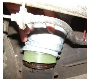
Fig 9 - Fabric duct slides over rubber bushing
