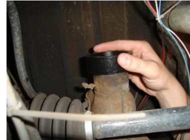
7a-Installing rubber boot onto heater box
