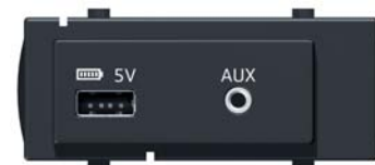
USB charging and AUX-In connector block
