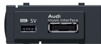
USB charging and AMI connector block
