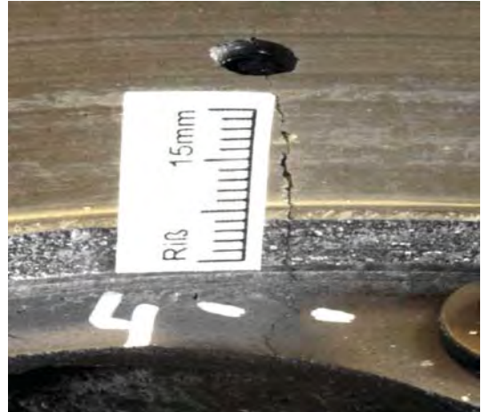
Critical interfacial crack propagation characteristic 441_028
