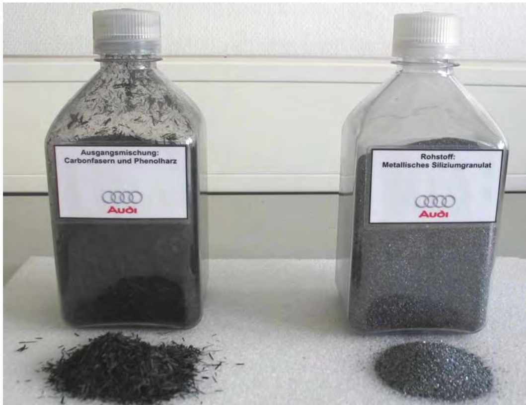
Primary materials: a compound of carbon fibres, phenolic resin and silicon granulate
