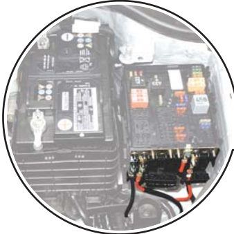
Back-up fuse box under the hood on the driverside
