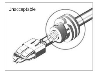
*e)* Also, check to be sure the crimp wings have not been over-crimped to the point of damaging the seal.
