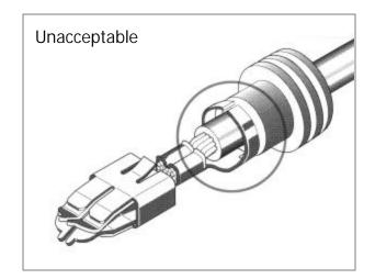
*d*) Check the crimp wings to be sure that the seal is well attached and secure, but not damaged in the sealing area itself.
