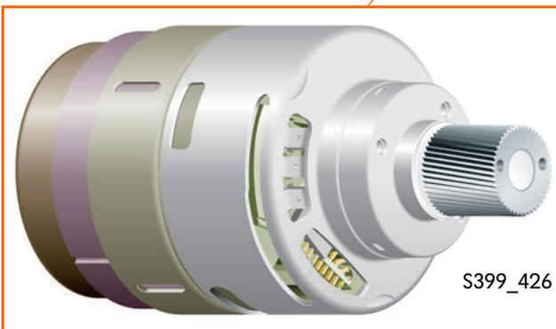
The electromechanical power steering motor V187 is mounted parallel to the rack in the steering gear housing. It transfers the steering-assistance force to the recirculating-ball gearbox via a toothed belt.
