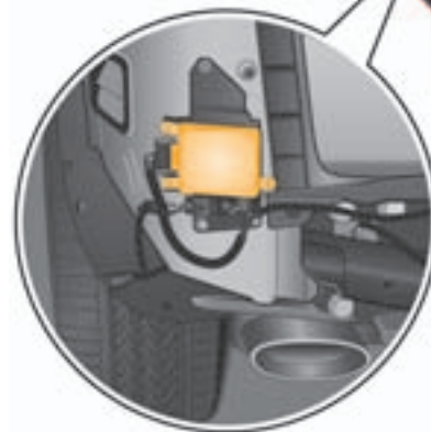
Lane change assist control unit J769 behind the bumper, left
