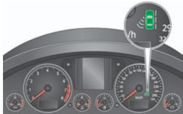
Lane change assist warning lamp K232
