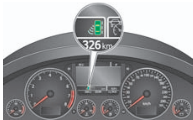
Lane change assist warning lamp K232
