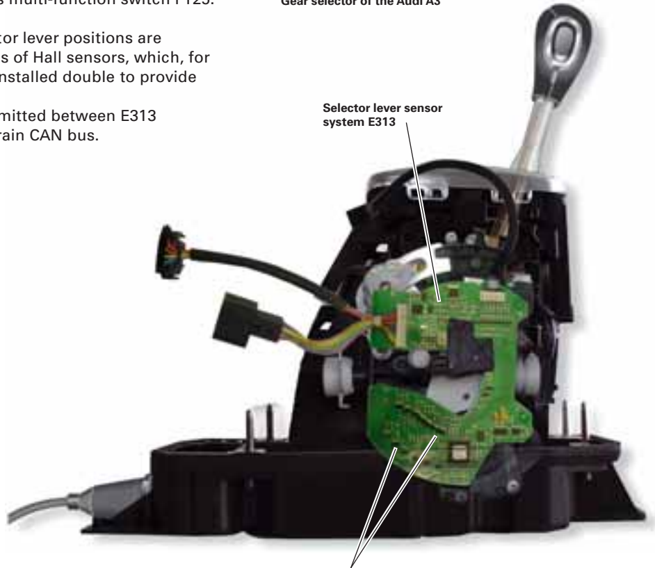
Hall sensors for determining selector lever positions P, R, N, D and S
