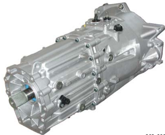
6-speed manual gearbox 08D/ ML400 (expected SOP: 2nd quarter 2006)
