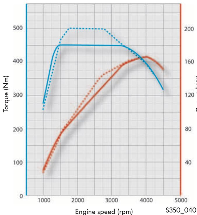
In the Phaeton, the 3.0l V6 TDI engine achieves its maximum torque of 450 Nm as of an engine speed of 1600 rpm; this is available over a wide speed range, up to 3250 rpm.
