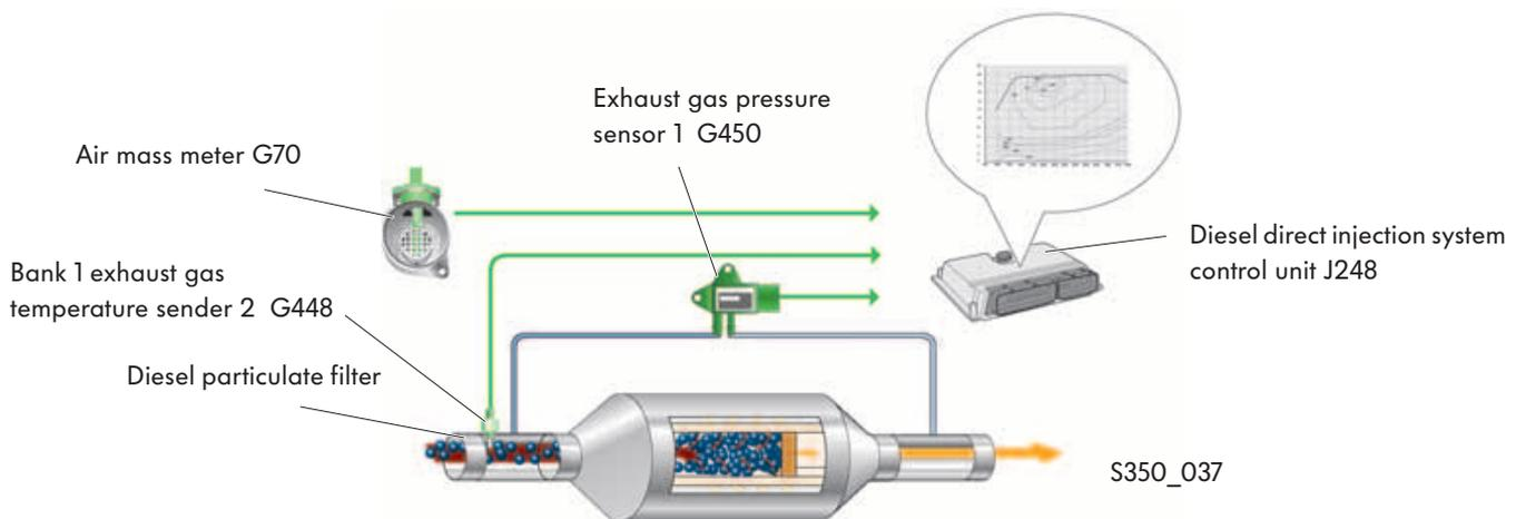
As soon as the carbon level limit value has been reached in the particulate filter, active regeneration is introduced by the engine management system. The following measures lead to a specific, temporary increase in exhaust gas temperature to approximately 600 – 650 °C. In this temperature range, the carbon collected in the particulate filter oxidises to form carbon dioxide.
