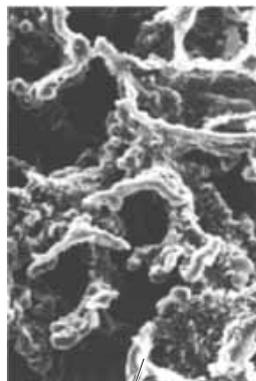
Cast iron with vermicular graphite
