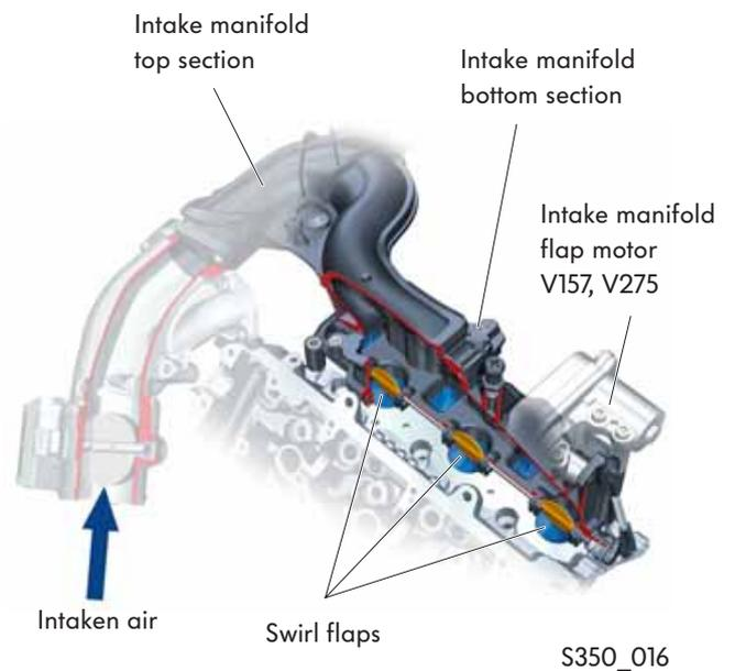
The swirl flaps are moved by the intake manifold flap motor via a push rod. To do this, the positioning motor is actuated by the engine control unit. An integrated sensor serves to feed back the current position of the swirl flaps.
