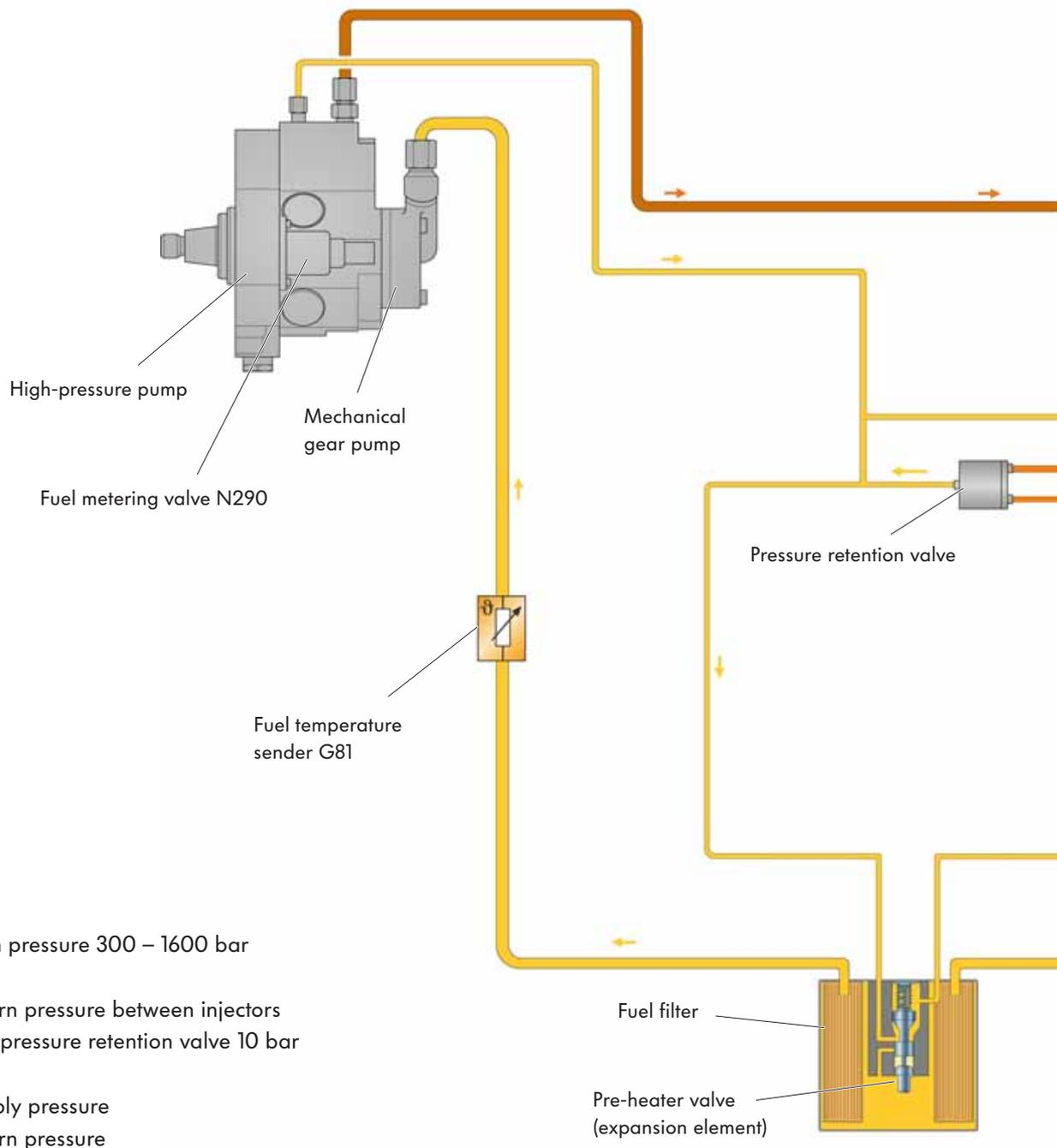
From the high-pressure accumulator, the fuel is forwarded to the injectors, which inject it into the combustion chambers.
