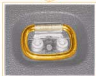
Lashing rings on floor
