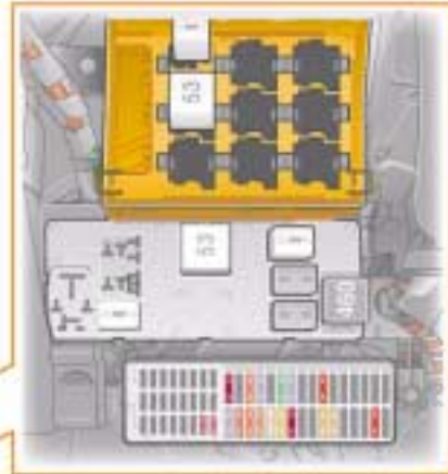
Relay carrier on left under dash panel
