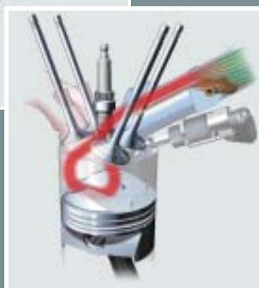
The 2.0 I 110 kW engine with petrol direct injection (FSI)
