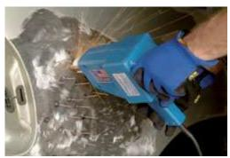
A newer and less invasive technique is to use a stud welder. It works by electrically spot welding 2mm-dia. copper-plated studs to the body surface. A slide hammer firmly grasps each stud and after a couple of sharp raps, the dent is out. Then, you twist off the studs and grind the surface flat. These welders cost about \$250 to \$300, and are sold at auto parts stores that carry body and paint supplies.
