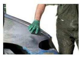
Click to enlarge **Wetsand again** to remove imperfections, including sanding scratches. There should be no bare metal showing.
