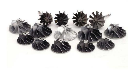
There are four TO4 turbine wheel trims (rear row)--N, O, P, and Q. The large Q-trim reduces backpressure, but being heavier, it spools up slower. Each trim level is available in two shaft diameters and with a choice of ball or plain bearings. In the front and middle rows are just 10 of the literally dozens of TO4 compressor wheel trims; they're ID'ed by numbers.
