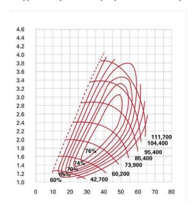
Chevy 350 (+0.030), Actual displacement: 355.11 ci, Peak engine speed: 6,500 rpm, Airflow: 1,349.15 cfm (94.44 lb/min), HP potential: 944 hp, Compressors: Two GT61 (47.44 lb/min per turbo), Approx. efficiency: 73%
