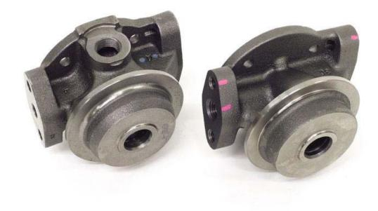
The little brother of the TO4 (far right) is the T3 (far left). The T3's envelope is about 25 percent smaller, making it easier to package. Turbonetics says many street V-8s run OK with T3 or T3/TO4 hybrids, which is a real godsend in a tight engine compartment.
