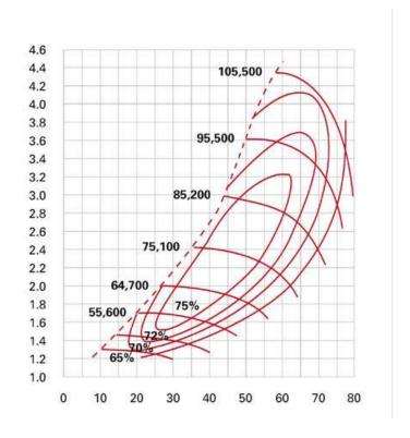
Chevy 454, Actual displacement: 453.96 ci, Peak engine speed: 6,000 rpm, Airflow: 1,592.01 (111.44 lb/min), HP potential: 1,114 hp, Compressors: Two GT70 (55.75 lb/min per turbo), Approx. efficiency: 70%
