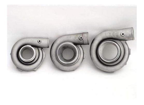
The compressor housing is a primary factor in determining how much boost (and power) a turbo is capable of supporting. There are at least nine different housings available for standard shaft-diameter TO4s alone! Here are three of 'em.
