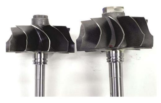
Turbonetics latest Inconel Super T turbine wheels (right) feature 10 improved high-efficiency blades in place of the previous 11-blade design. Super T turbines fill the gap between the TO4 family that tops out about 900 hp and the huge Super Thumper family that starts working at 1,400 hp. Inconel is good up to 1,700 degrees F. Need more? Special Mar-M 247 exhaust wheels survive at 2,000 degrees.
