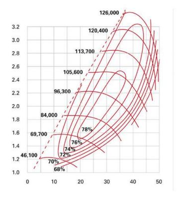
Honda B18, Actual displacement: 1,834 cc (111.95 ci), Peak engine speed: 9,000 rpm, Airflow: 588.88 cfm (41.22 lb/min), HP potential: 412 hp, Compressor: TO4E-50 trim, Approx. efficiency: 72%
