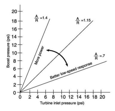
For any turbo series, the higher the A/R ratio, the better the top-end performance. The lower the A/R ratio, the better the low-speed response.
