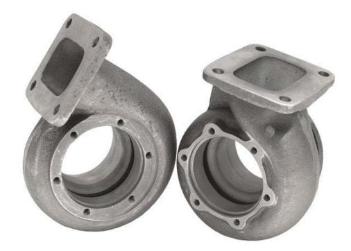
A tangential turbine housing (left) offers about 4 percent higher flow but has less mounting and packaging
