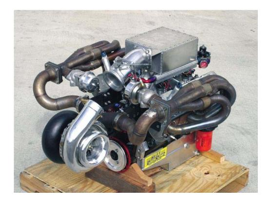
This 358ci small-block Chevy is about as rad as it can get and still use conventional 23-degree-valve-angle heads. Electronically managed by ACCEL Gen 7 DFI, the 10.0:1 engine runs a single large-frame Innovative GTB88 turbo and makes over 1,400 hp on C-16 race gas. Big race turbos are typically identified by the inducer orifice size--in this case 88 mm.
