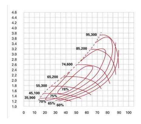
Ford 302, Actual displacement: 301.59 ci, Peak engine speed: 6,000 rpm, Airflow: 1,057.67 cfm (74.04 lb/min), HP potential: 740 hp, Compressor: GT76, Approx. efficiency: 66%
