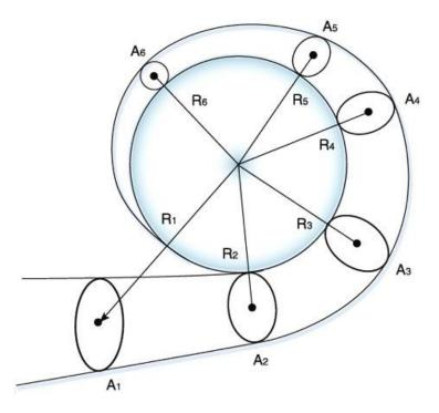
The turbine housing A/R (area/radius) ratio is the area (A) of any turbine inlet scroll cross-section divided by the distance from the center of that cross-section to the center of the turbine shaft (R). For any given turbine housing, A and R vary in the same proportions, so all As divided by their corresponding Rs yield the same dividend--which is the A/R ratio.
