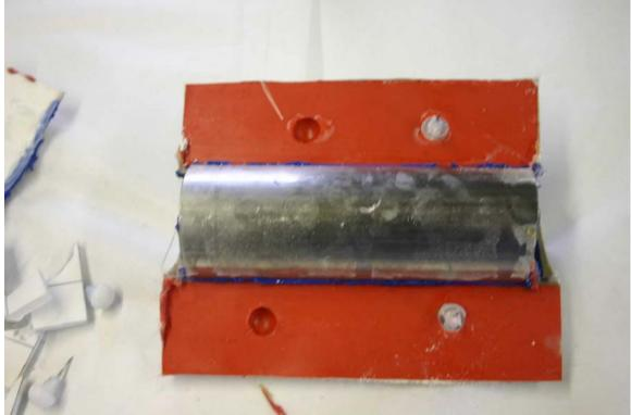
Don't loosen the metal tube. Now wax the tube and flanges with six coates of wax and PVA. Repeat laying on two coats of gel coat followed by the
