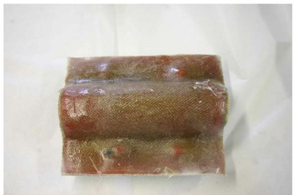
The part after six layers of 6oz. Cloth and allowed to dry. The next step is to flip it over and remove the foam board support and flanges and clay. Pop out the plastic buttons.
