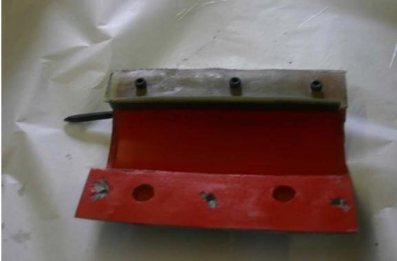
Bolt the lip to the mold half. Again wax and buff. Begin laying down a layer of resin followed by a layer of CF. I used fiberglass to backup the CF just to save materials for this
