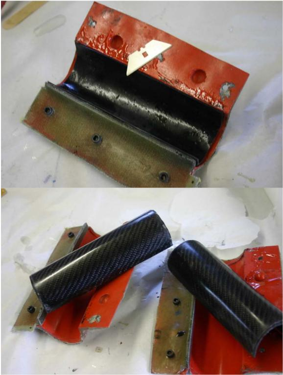
You can now sand the lips on each finished piece and bond together with resin or use an epoxy glue for strength. A better way which everything in perfect alignment is to unscrew the lips from the flanges. Wax the mold and replace the CF half tubes. Run a small amount of resin along the lips and then clamp the two mold halves together. I then saturate fiberglass tape and place the tape over the inside lips to
