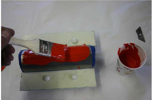
I apply this in two coats to about 1/16<sup>th</sup> inch thick and allow to dry to fingerprint dry state. Its then time to start laying on the fiberglass. I use chopped fiber for the tight places and around the plastic
