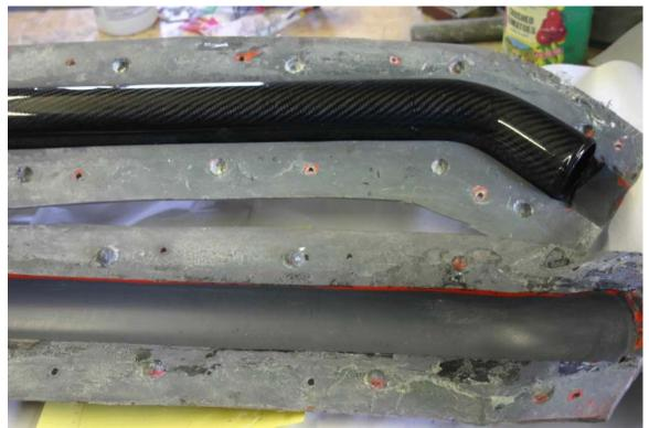
I'm also using a bit different technique to make seamless tubes using CF sleeves and an inflatable blader. I hope this helps with your future project.
