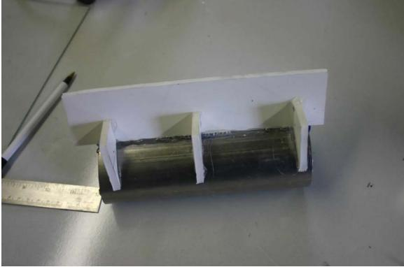
The flanges are waxed on the side to be molded and also sprayed with PVA. Once its all dry its time to apply the gel coat.
