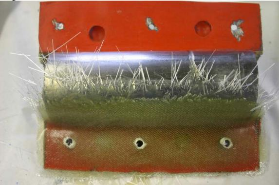
Once dry, remove the tube and trim the raw edges to about <sup>3</sup>/<sub>4</sub>" wide.
