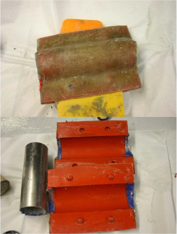
Remove the tube, wash off the PVA with water and then wax the mold. Note how the plastic rounds allow perfect alignment. This step is only necessary for tube. You need to form an inner flange to allow the final tube halves to be bonded.
