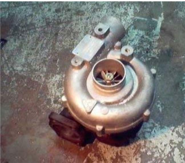
This is the KKK Turbocharger, The KKK turbo comes from Germany, many European cars use these turbos. Audi/VW/Porsche and others. This turbo shown the KKK 26 I believe, is similar to a basic T-3 turbo. The inlet flange is identicle to the T-3 turbo. But some other KKK turbo's have very odd looking inlet flanges.
