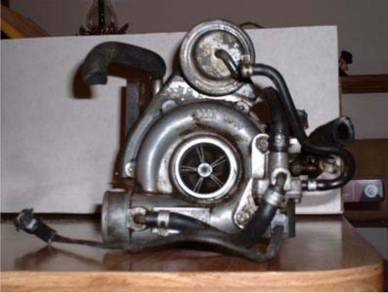
The IHI RHB5 Turbo, a few different styles of this turbocharger, This turbo is the Ford Probe/Mazda MX6/ 626 Turbocharger. It has a circular inlet flange, and wastegate that is set at 8psi.
