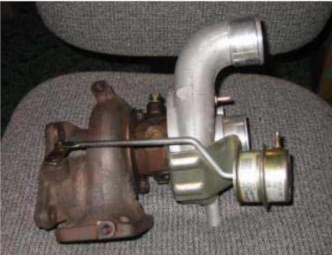
The 2g DSM T-25 turbocharger. This was the first turbocharger I ever worked with on a Custom Project. It is Oil & Water cooled like the 14b. The 14b & TD04 are Mitsubishi Turbos, The T-25 Turbo is made by Garrett.
