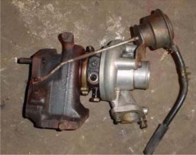
Next up, is the little guy, The DSM 1g Automatic Turbo. Known as the TD04. The TD04 is basically shaped the same as the 14b in most ways. The exhaust wheel and compressor are a bit smaller. This turbo boost's similar to the DSM T-25 turbo setup.
