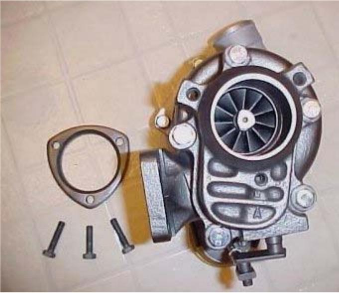
This is a basic T-3 exhaust housing flange with an internal wastegate. One of the easiest to make a downpipe with. All you do is bolt that flange to the housing, and take it to an exhaust shop to make your downpipe... Simple Simple..
