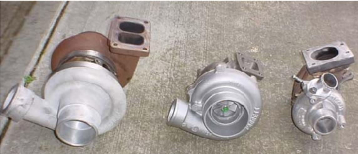
T4 Turbocharger (Diesal Truck) - T3/04e Turbocharger - 14b DSM Turbocharger
