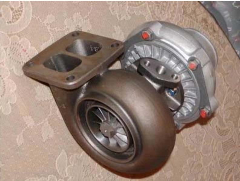
The Big Bad Boy Turbo, T4 turbo. There are many series of these turbos, I am not familiar with that many of them, since I have never used one. These are for very large HP applications. Mainly v6 or v8's. Some heavily built race Honda B/D series motors can be used with these, mainly for drag racing.
