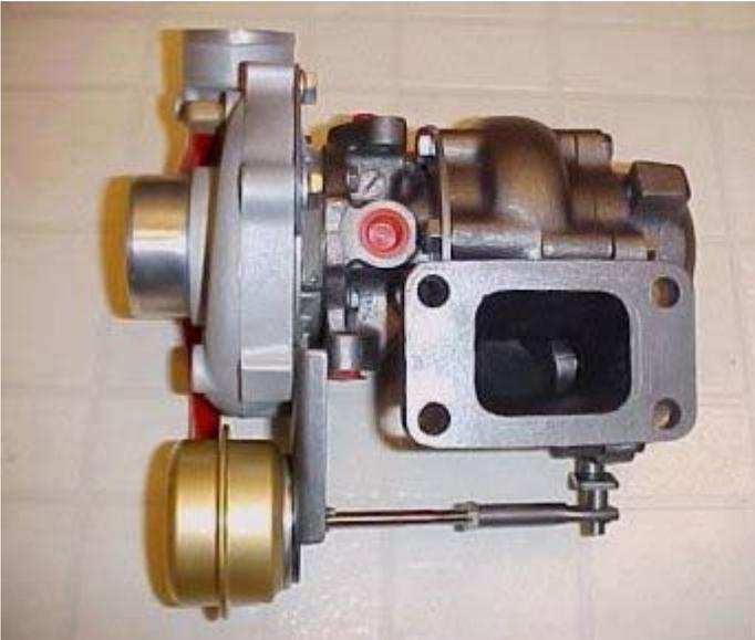
The T-3 Turbocharger. This is the standard in most turbochargers. Garrett T-3 turbo's are used in lots of Factory cars. First off how to identify a T3 turbo. All true T3 turbochargers have a rectangular flange with 4 bolt holes. For compressor housings and exhaust housings, their are just so many different styles and combinations. .48 a/r's all the way to .82's
