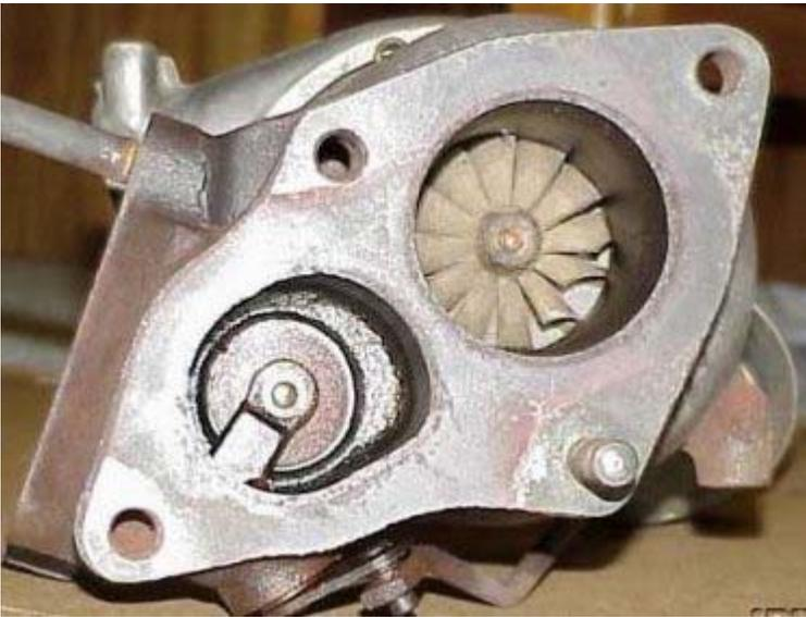
This is what makes the 14b such a great turbo, the exhaust wheel is one of the largest for a factory Turbo'd 4cyl cars. You can see the wastegate flapper to the left.
