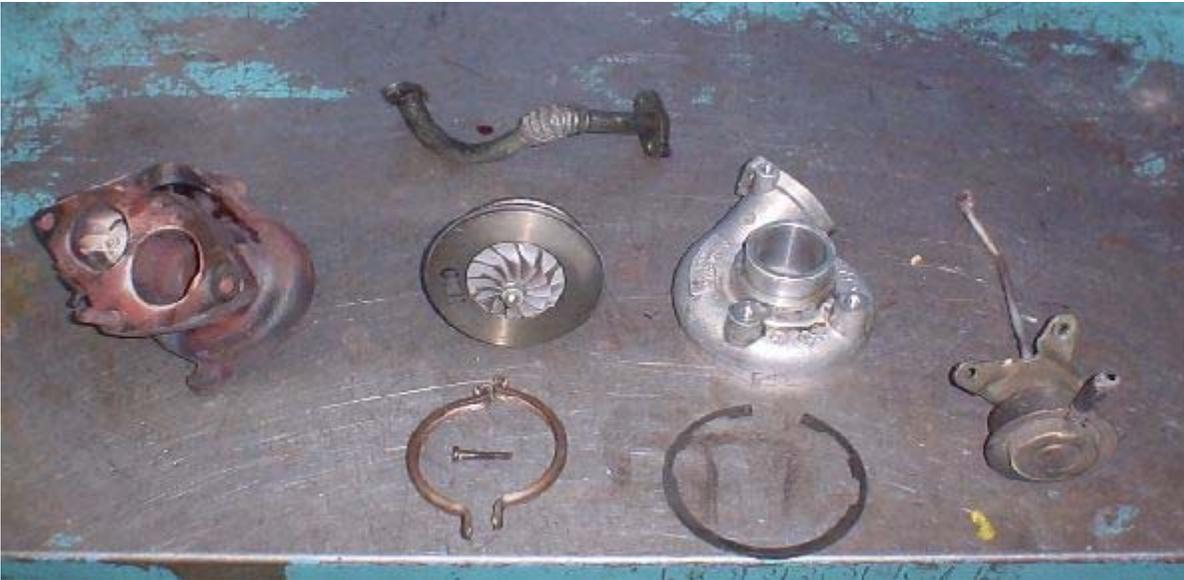
Exhaust Housing - Turbine (center section) - Compressor - Internal Wastegate
