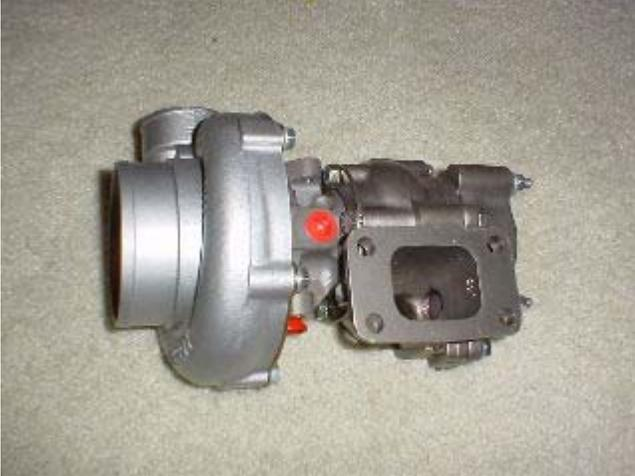
Hybrid Turbochargers, T3/T4 Turbos... The concept of using a small center section to spool fast and using a large Compressor for more cfm. These turbos are one of the best to use. Especially on B-series Motors. T3/T4's can support anywhere from 300-450hp. Some can come internally gated or external. This is a .70ar compressor .63 exhaust
