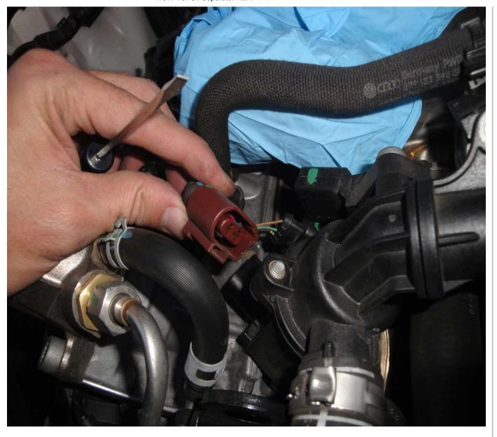
Step 6: Using a screwdriver and some anger, remove the clamp from the turbo inlet-to-bypass valve on the driver's side. Then, remove the <u>bypass valve assembly</u> from the driver's side:
