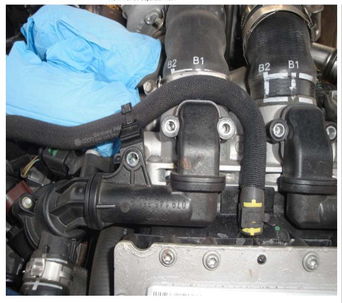
Step 3: Do the same for the passenger side. Insert shop towel to ensure no debris goes into the holes:
