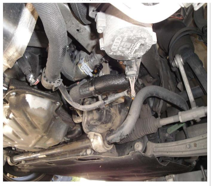
Step 23: Loosen the outer <u>brackets</u> from the lock carrier to the fender support thing on each side:
