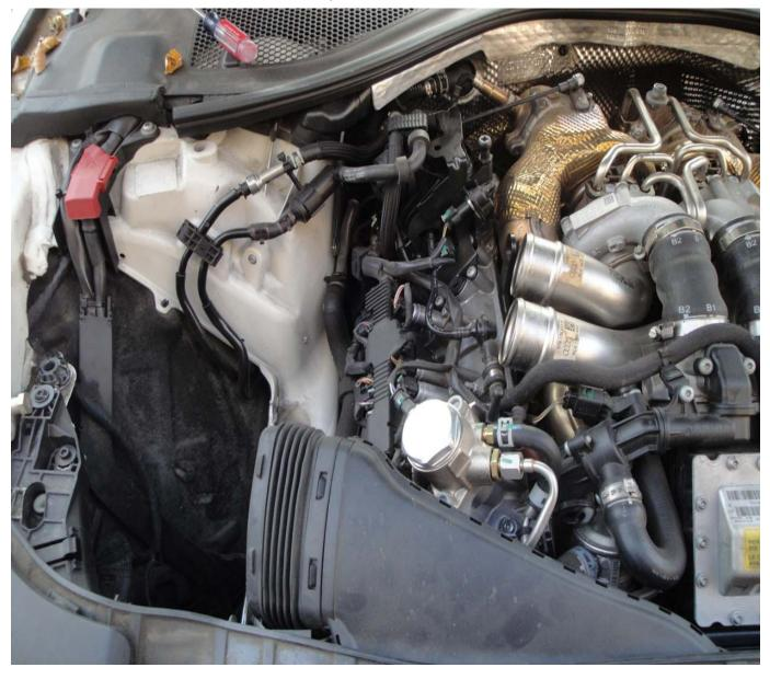
Step 2: Use compressed air to blow off the throttle body area of debris. Using a T30 Torx, remove the three bolts from the driver's side bypass valve-to-throttle body connection (The longer bolt goes on the outside):
