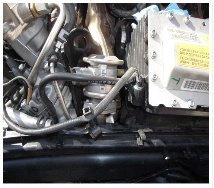
Step 37: Using a T30 Torx, remove the 6 bolts (3 per side) that connect the intercooler runners to the intake manifolds. One is on the top, another is on the outside bottom, and one is about 3 inches inward from the second <u>bolt</u>. A carrier will come out with the <u>bolt</u>, don't worry about it:
