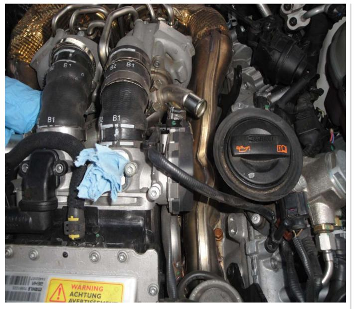
Step 7: Remove the <u>clamp</u> holding the passenger side wastegate hose to the intercooler. Remove the hose and push it off to the side:
