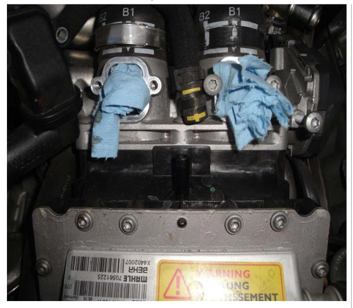
Step 4: Using a 7mm nut driver, loosen the <u>clamps</u> on the turbo-to-throttle body <u>tubes</u>.
