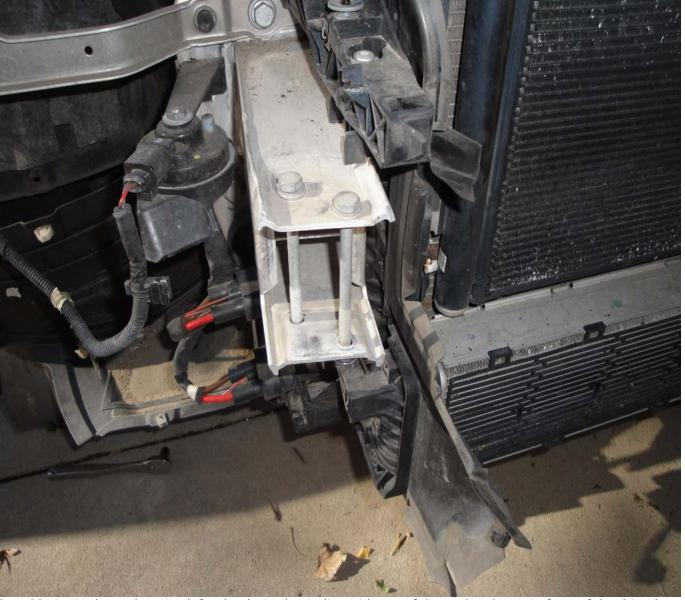
Step 22: Drain the coolant. Look for the drain plug in-line with one of the coolant hoses in front of the driver's side <u>wheel</u>. About 2 gallons will come out. Be sure to completely remove the plug for faster draining and open the expansion tank lid for venting:
