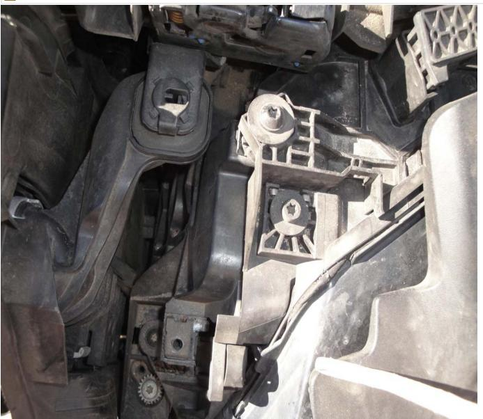
Step 16: Gently pull on the rear edge of the bumper where it meets the fender outwards, until it becomes dislodged. Do this on both sides.
