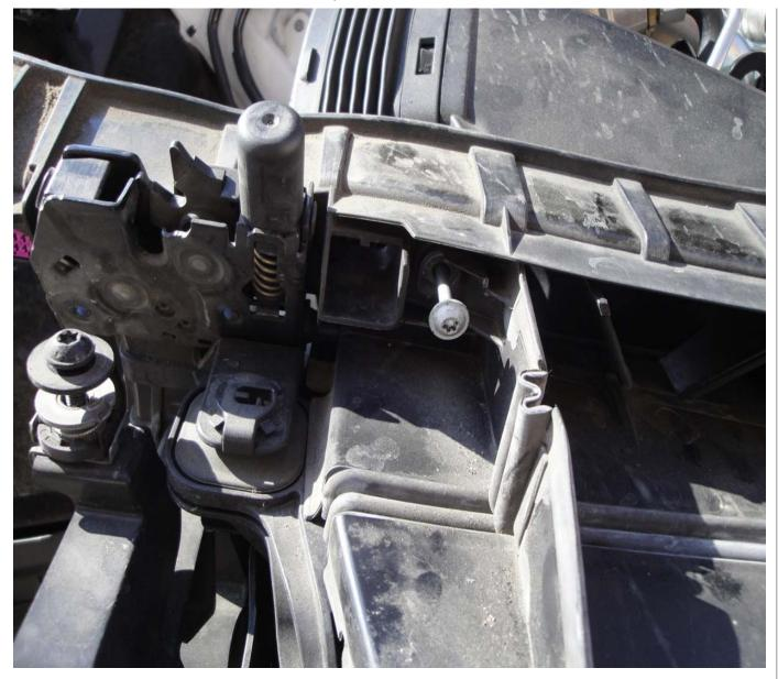
Step 30: Remove the  $\underline{\text{coolant}}$  hose clamps on the  $\underline{\text{intercooler}}$ . Disconnect the  $\underline{\text{hoses}}$  and push them off to the side:
