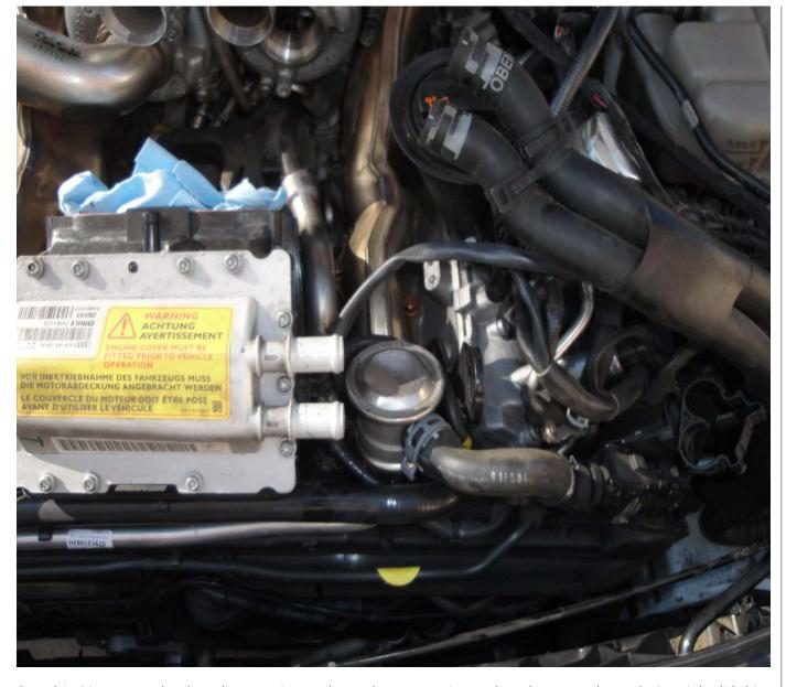
Step 31: Disconnect the three hoses going to the coolant expansion tank and remove the tank. I mainly did this to gain access to the <u>spark plugs</u> (highly recommended during this <u>repair</u>).
