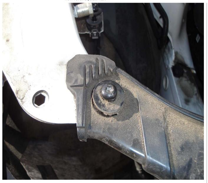
Step 27: Using a 16mm socket with extension bar, remove the 3 bolts on each side that attach the <u>lock</u> carrier to the frame rails. While the <u>lock</u> carrier won't fall forward due to the <u>radiator</u> hoses still being attached, I wanted to make sure it was supported and not dangling from any hoses/wires. Use a jack stand or two to support it and slide it forward:
