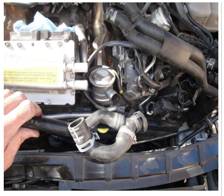
Step 33: Using a T30 Torx and extension, remove the <u>bolt</u> holding the coolant crossover tube on the driver's side head. Remove the clamp on the passenger side and remove the pipe altogether:
