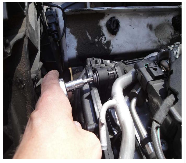
Step 38: Using a 5mm Allen with extension, remove the three bolts that hold the <u>intercooler</u> to the block on either side. It looked like there should be a 4th bolt on the driver's front, but there wasn't:
