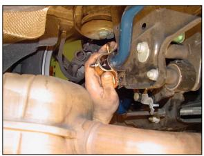
9/ Re-install the end link bolts and nuts and leave loose. Secure the bushing brackets. Tighten the four bracket bolts, then tighten the end link bolts.
