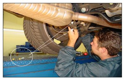
5/ Remove the two end link bolts and nuts (16mm wrench) which attach the bar ends to the end links and save them. To clear the shocks with the bolts, pull the bar towards the rear of the car.
