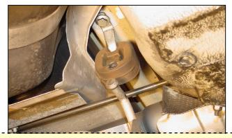
This document was created by Print2PDF http://www.software602.com 4/ Remove the four bushing bracket nuts and bolts (13mm wrench) attaching the anti-roll bar brackets to the sub-frame and save.
