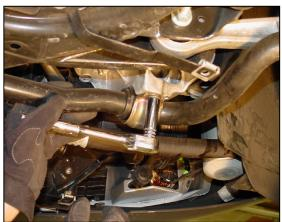
5/ Apply a quarter tube of grease to each inner-channeled portion of the two new front bushings and attach to HSport bar against the outside of the washers on the bar. Slip the new brackets over the bushings.
