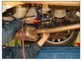
\*Adjustability Note: To adjust between the two holes, you must unbolt the bushing bracket bolts and pull the bar towards the rear so that the end link bolts clear the shock bodies. The hole at the bar's end is the softer while the second hole from the end is the harder setting.
