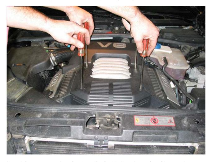
Step 1 is to remove the trim, then the intake hose from the airbox to the throttle plenum. Remove the 2 10mm bolts that hold the intake plenum onto the throttle body. Once removed, the plenum will slide to the rear, and be free of the throttle body. It is not necessary to remove it completely from the car. It is a good idea to carefully remove the breather hose from the passeger side valve cover, just to get it out of the way. (Squeeze the end, and wiggle it free) Unplug the harness connector
