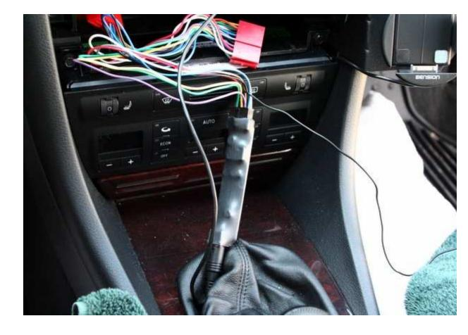
11) Wire the grounding cable from the IceLink wiring harness to the grounding point on the  $h\epsilon$  unit:
