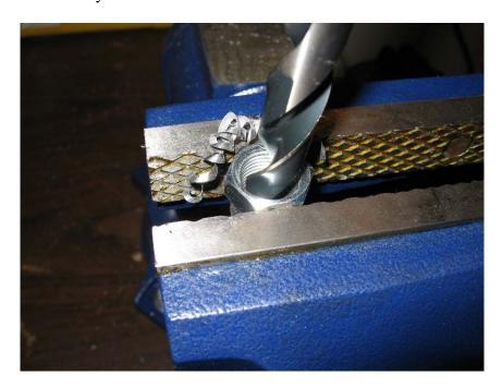
The O2 sensor goes into the drilled anti-fouler
