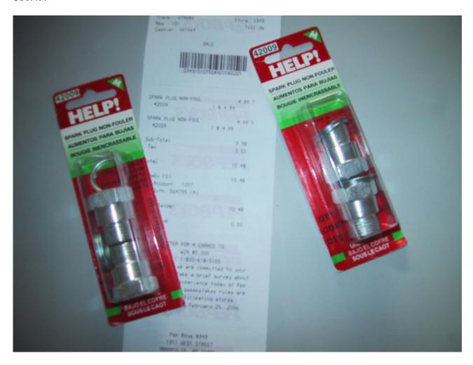
You have to stack two to make it work. The first one has to be drilled out to 19/32" which is the size of the O2 sensor body:
