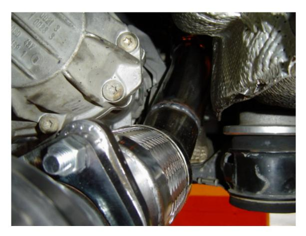
Make sure you have enough clearance for the O2 sensors, about .5" should be good to compensate for any possible exhaust movement.
