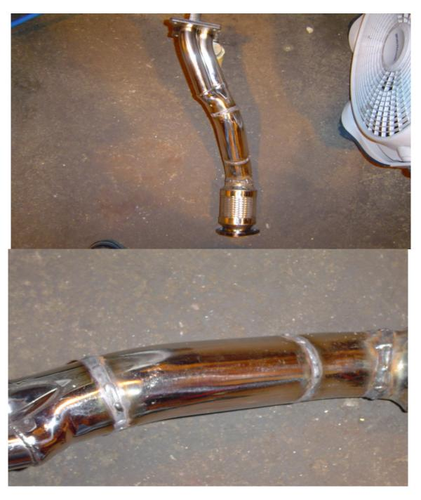
Make it a straight cut if possible so you can turn the cut out middle piece of the pipe for appropriate adjustments. Bolt on the DP header of the pipe to the Turbo, hold the cut out pipe in the place where you want them, use a black marker to mark their new, to be welded position. That was easy, wasn't it;-)
