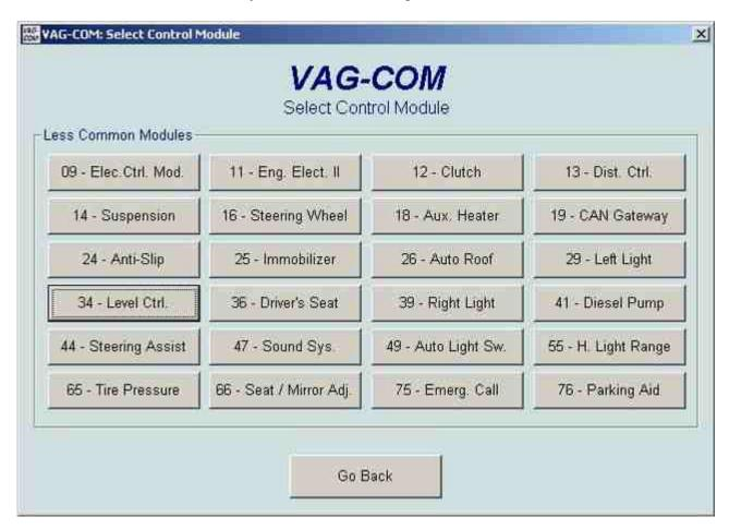
Click on Module 34 to enter the Level Control module. Your VAG-COM will open the module and you'll be presented with this screen. Click on Advanced Function 11 for the Login screen. This function unlocks the adaptation module.
