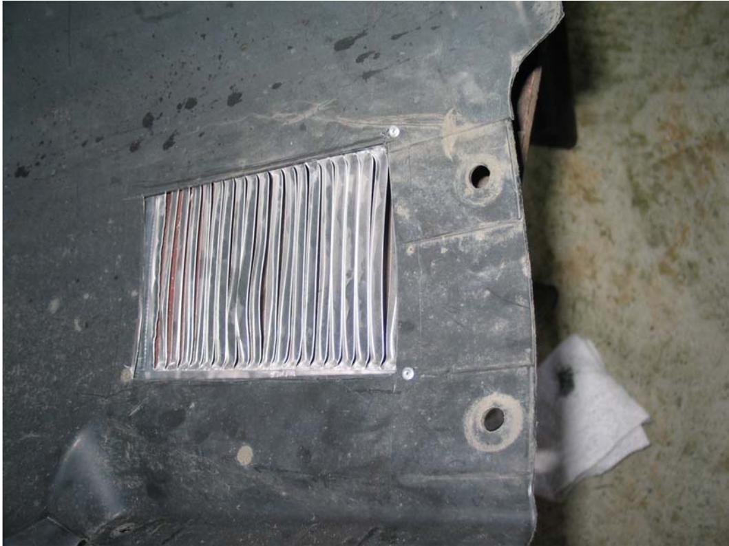
Three more on each side and one at the bottom and you are all set. I also put a dolly under the rivets and hammered them down a little more with a punch, but this is not necessary if your rivets look "toyt". Mine did not all around. The top did not need a rivet as the liner bends and closes the gap just fine. Feel free to add one if you like.
