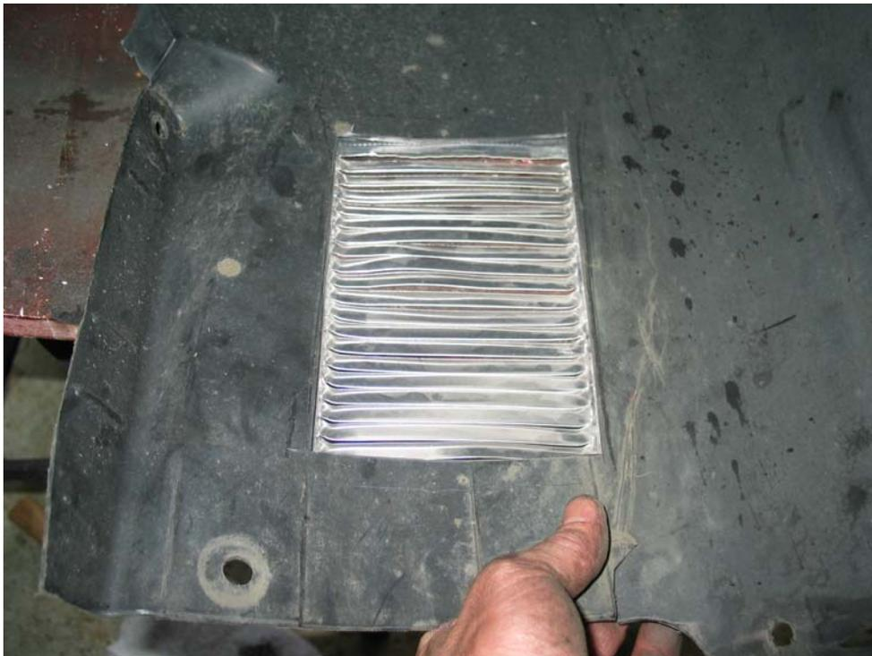
I held the grate in place and drilled the first two holes. Popped two rivets in and continued all the way around.
