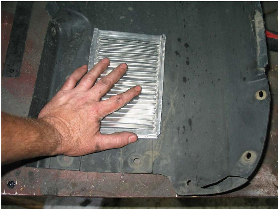
Mark the outline of the grate on the fender liner with an angled pencil. All the way around the grate so the hole would be the size of the grate.
