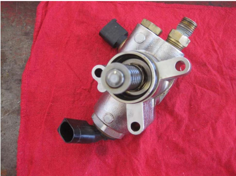
16. Per Bentley manual it is recommended that you replace the round fuel pump seal. The following photo shows the seal to be replaced. Audi part number for the seal is 06E 127 248. It costs \$9.68 from my dealer.
