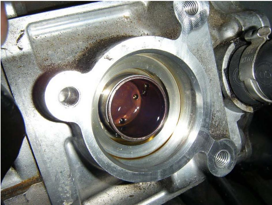
18. Place the three torx bolts into the pump and set the pump in place to be secured. Once the pump is fully seated and all three bolts are in finger-tight, use a torque wrench to tighten them evenly to 10Nm or 7.4lb-ft. The bolts are quite long; over-tightening them could stress them and cause a failure that would put the pump on quite a bind. If you are unsure about what torque the bolts are in, remove them one at a time and re-torque them to make sure.
