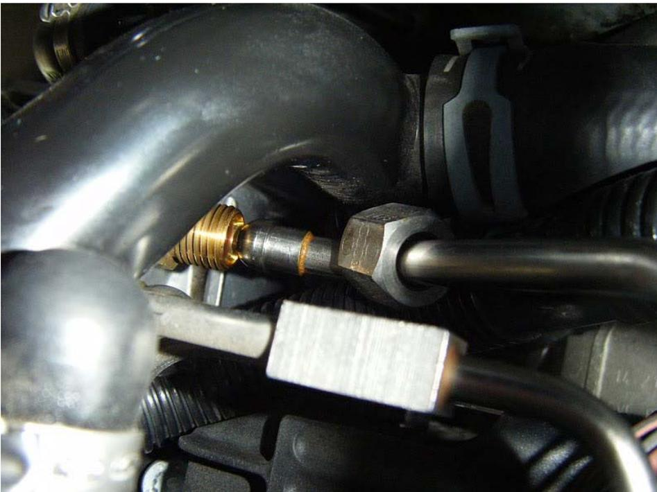
10. Now, using 12-point 8mm torx bit remove the banjo bolt from the pump
