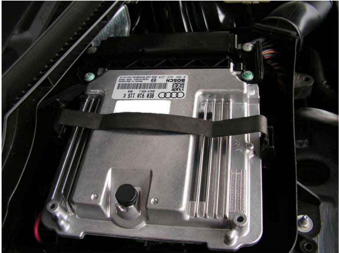
By removing the spring strip you now can move the ECU around as the cables connected to it have a bit of slack.
