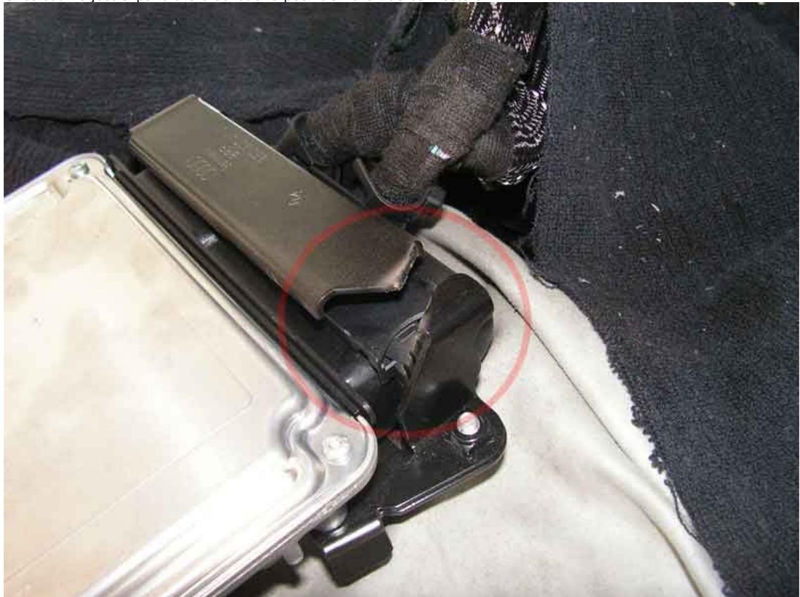
Unplug the connector (by pulling a small flap outward on each side) and your done.
