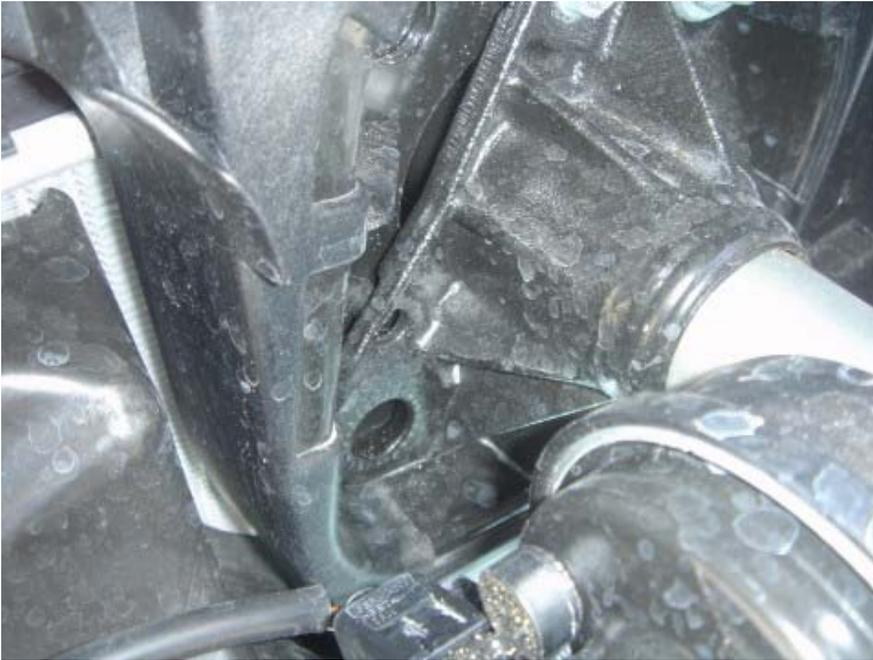
3. Locate OEM Snub beneath engine bay (adjacent radiator wall).
