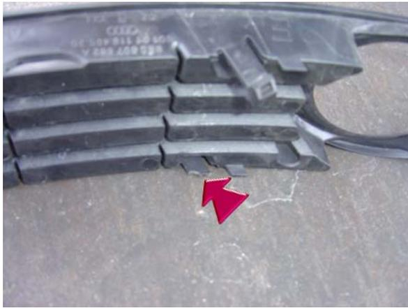
46. Trim the lower clip on the lower part closest to the fog light opening on both the passenger & driver side inserts.
