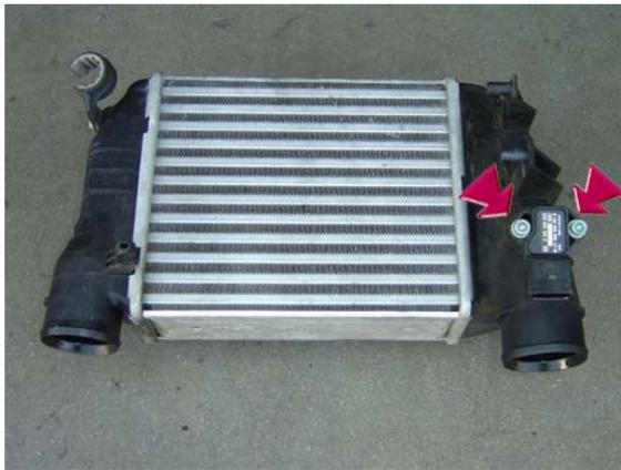
26. Remove sensor from stock intercooler and place it in a safe location for use at a later step.
