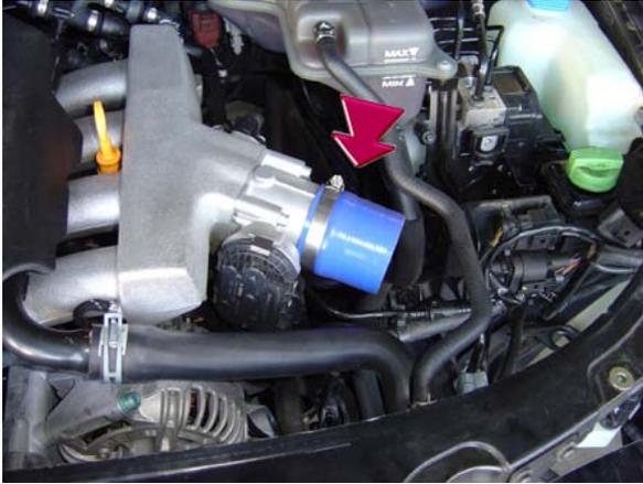
40. Slip the 2.5 silicone hose onto the throttle body and secure in place using of two larger hose clamps supplied with your kit.
