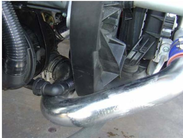
38. Slip a clamp over the passenger side silicone hose and install the intercooler piping as indicated by the images. Before tightening the clamp rotate the pipe as clock wise as possible to gently push up against the smog pump. Have someone hold the pipe in place pushed up against the smog pump while you tighten the clamp on the silicone hose.
