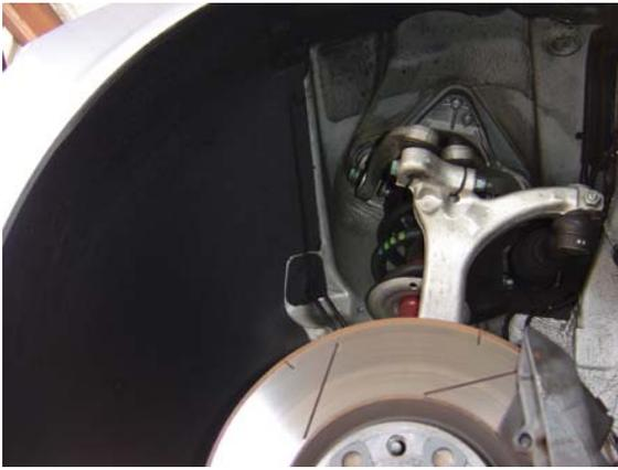
28. Remove the driver side wheel and undo screws that hold the fender liner in place.
