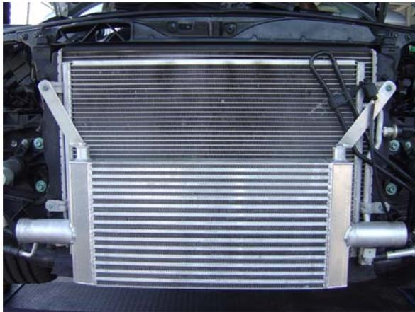
36. Slide the supplied lock washers onto the intercooler bolts and attach the intercooler to the support brackets. Tighten the upper AC condenser mount and intercooler bolts. By grabbing each end of the core gently lines up the FMIC using the fin lines on the AC condenser try your best to center the core as well.
