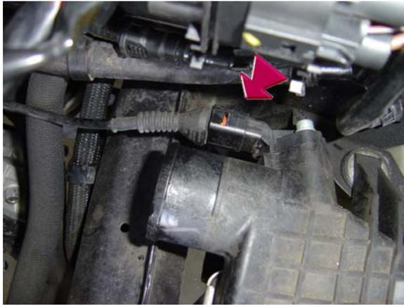
24. Disconnect the intercooler sensor.
