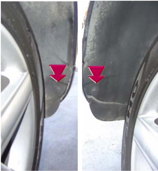
6. Remove the outer most screw on both the drivers and passenger fenders as indicated in the image. Turn the steering wheel to the left/right to assist.
