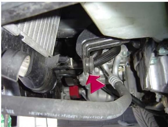
23. Slide the bottom of stock intercooler forward by pushing it out of the rubber mount.
