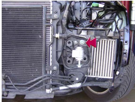
20. Remove the 3 torx 45s from around the bumper supports. Put one of the screws a few threads into the open service position. Repeat this on the passenger side as well. Pull the entire assembly forward. It will slide back 2 inches, and the weight will be supported by the service position screws. Do not put any additional weight on the assembly.
