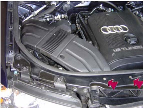
8. Remove screws for airbox channel & remove the channel.
