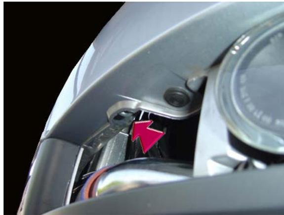
13. Using an allen wrench, loosen the two main bumper support bolts.
