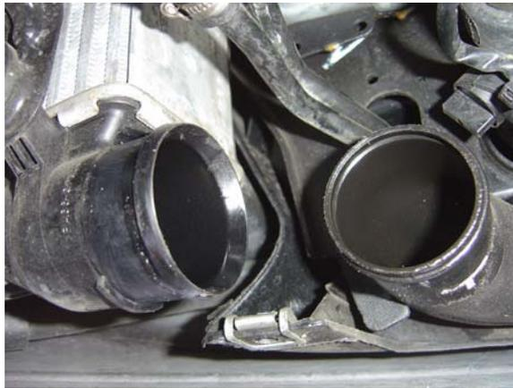
5. Disconnect and remove 90° elbow from the drivers side stock intercooler piping.
