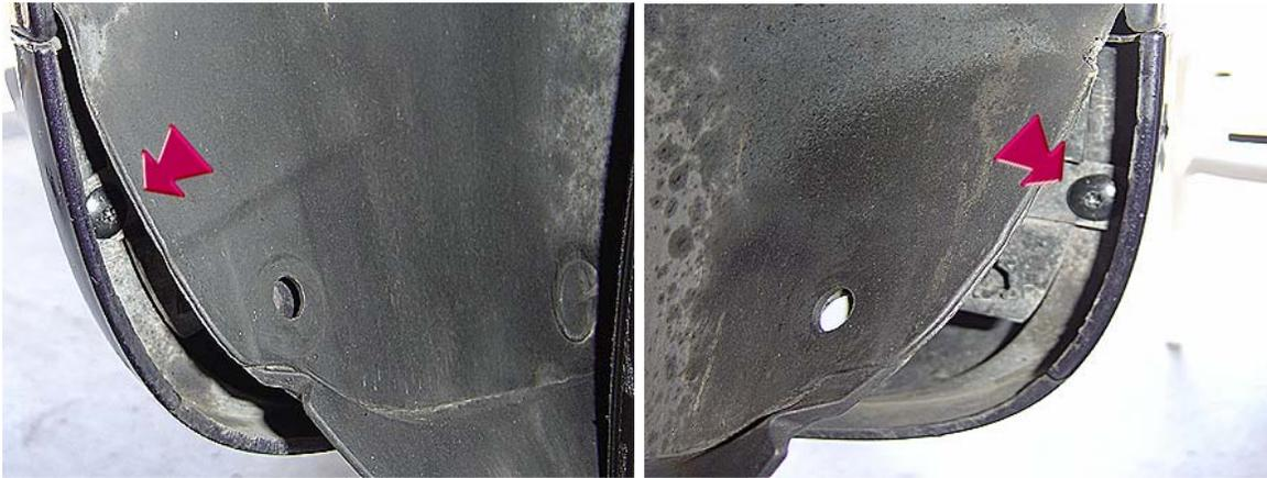
7. Lift the fender liner on both the drivers and passenger side and undo the torx screw underneath.
