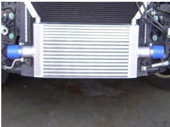
37. Slide the 2" silicone end hoses on. Use hose clamps to secure.
