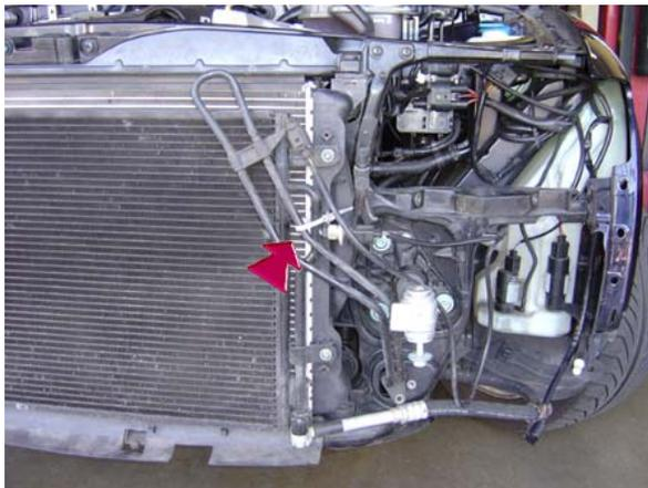
34. Insert the power stirring cooler back in its mounting hole and rotate it in an upright position against the air conditioning condenser as shown in the image above. Using the supplied zip ties secure the power steering cooler in place. The arrow shows and example of an area that can be utilized.
