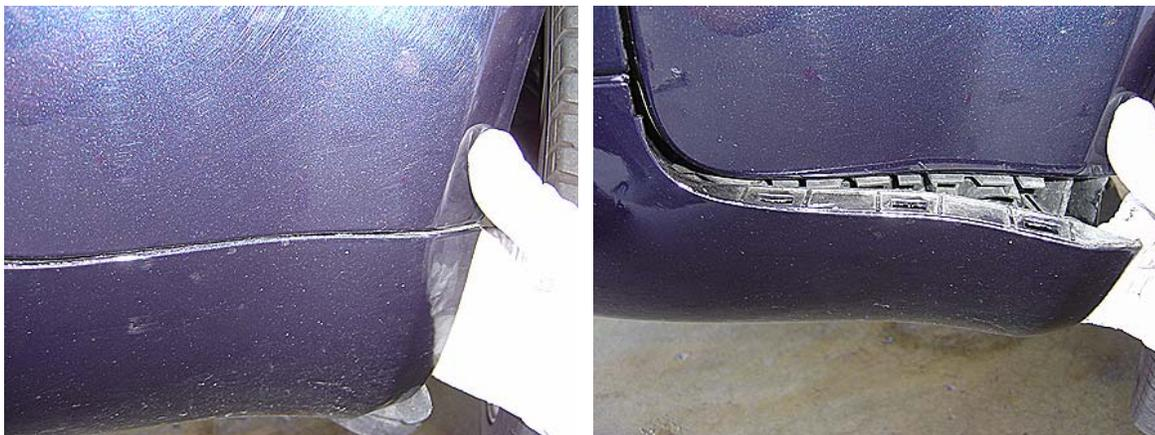
11. Gently pull outward to separate the lower bumper trim from the fender on both sides.
