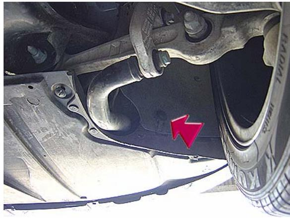
1. Remove the inner two screws on the inside of the fender liner, on both the left and right side.
