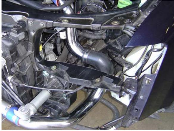
44. Attach lower intake pipe to the intercooler, line up the two intake pipes up and connect them together with the supplied 90 degree elbow. Be sure to tighten all hose clamps.
