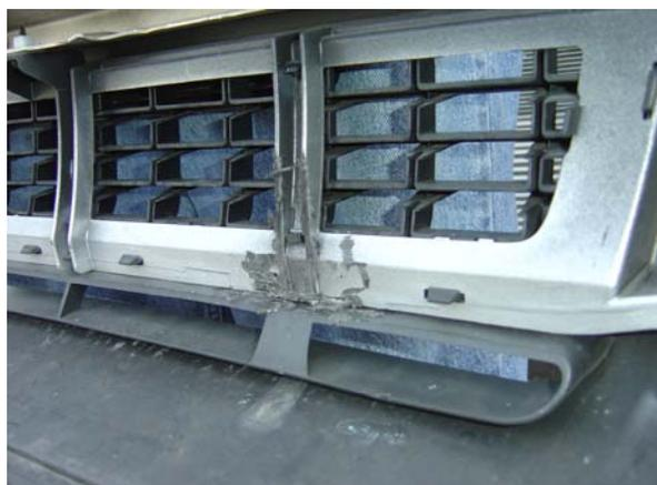
45. Using a rotary tool trim off the two areas indicated by the arrows.
