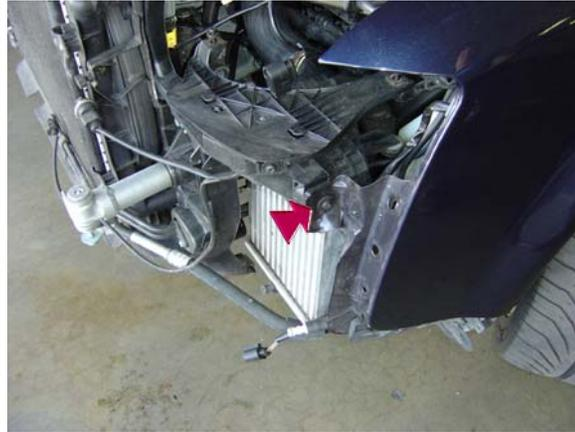
19. Remove the torx 30 screws on the top, and torx 30 screw from the side complete this on both the drivers and passenger of the car.
