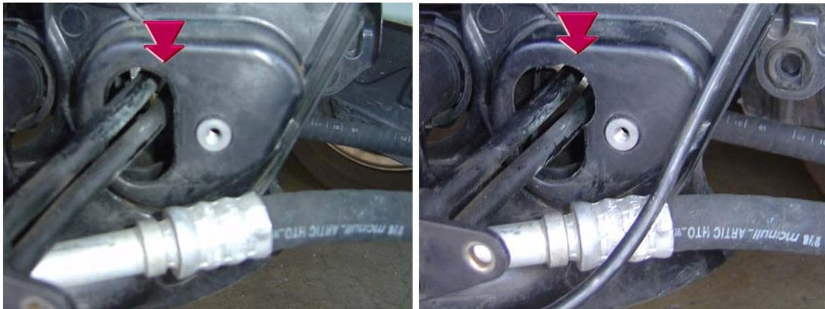
33. Use a rotary tool to enlarge the top portion of steering pump hole.
