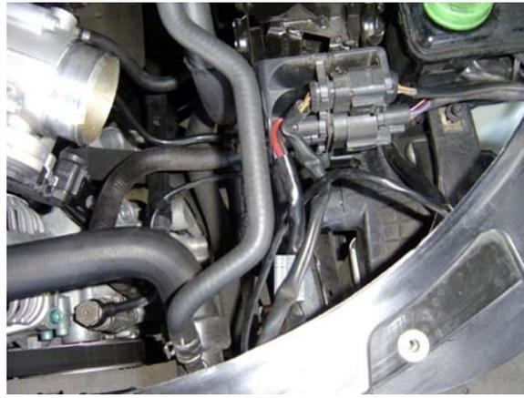
18. Remove the hose between the stock intercooler and intake manifold.
