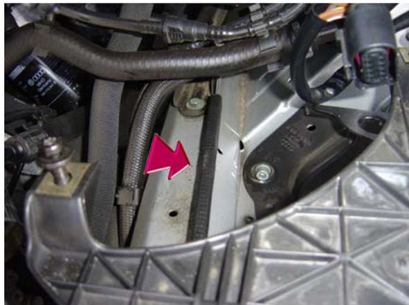
42. Slide the supplied pinch molding on the seam that runs underneath the driver's side headlight tray.
