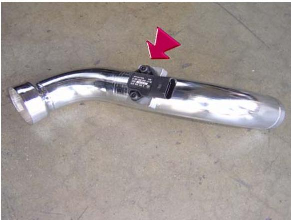
41. Attach the intercooler sensor to the flange located on the metal intake piping using the supplied black allen screws.
