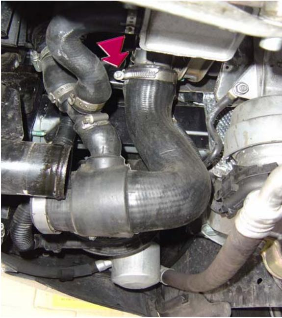
4. Loosen the clamp connected to the turbo outlet hose. Rotate it counterclockwise to relieve the tension. Do not disconnect.
