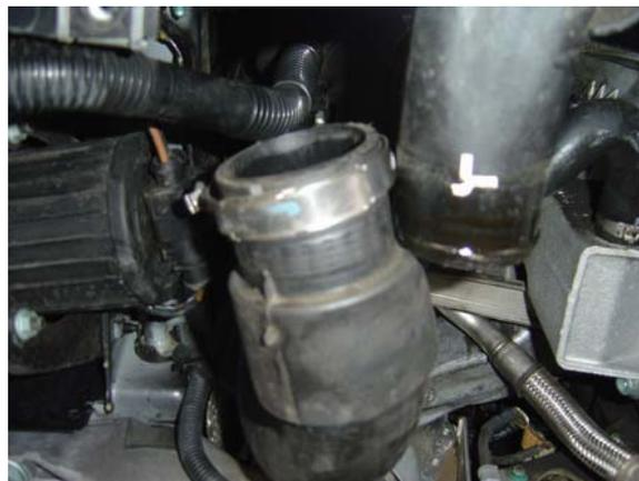
3. Disconnect the turbo outlet hose that is connected to the stock intercooler piping and move it to the side as shown.
