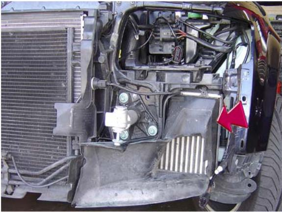
15. Remove the stock intercooler duct.
