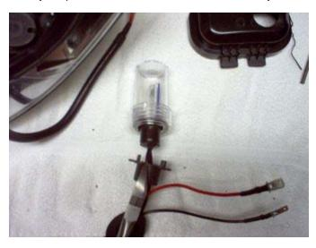
8. Feed the AMP connector ends of the bulbs through the hole from the inside out and seat as shown. Seal the provided 1" gasket in the hole you have made. You should have two connectors coming out of the same side as the bulb that will eventually connect to the OEM harness - these will be connected later. Leave the bulb in the case for
