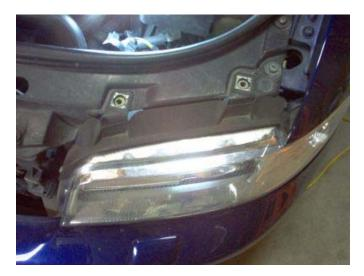
4. The third screw is shown here. A long extension is needed to get to it and an extendable magnet is helpful to retrieve the screw (or bit if it falls).
