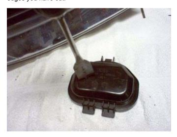
7. Some of the bulbs come with adaptors that some other cars require. The Audi installation does not require them. Take your pliers and cut them off. This will allow you to remove the base of the bulb case later on.
