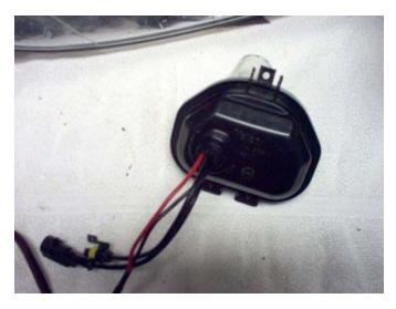
9. Now mount the ballast to the underside of the headlight housing with the double-sided tape provided. The square opening is perfect to mount the ballast to but other locations are possible also. There will be extra wiring so try to tie it up out of the way.
