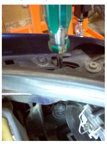
5. Disconnect the headlight and turn signal connectors and remove the headlight by pulling it toward the outside of the car and toward you.
