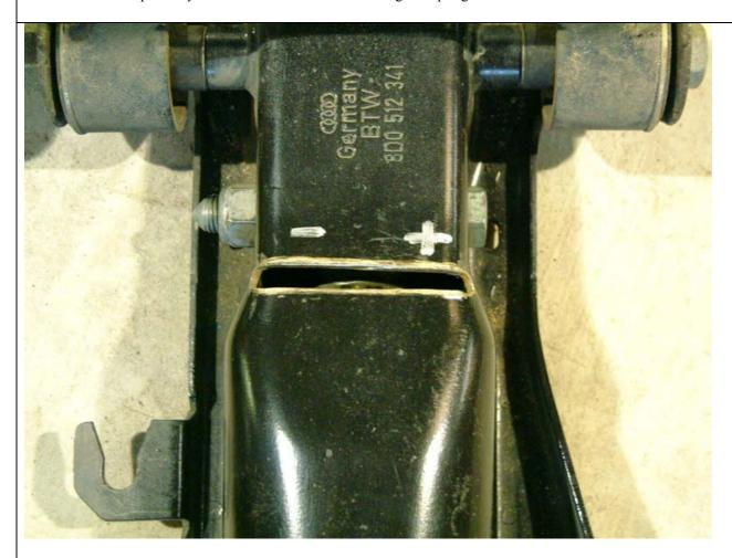
Once the slot has been complete, spray the slot with some type of anti-rust corrosion resistance spray.
