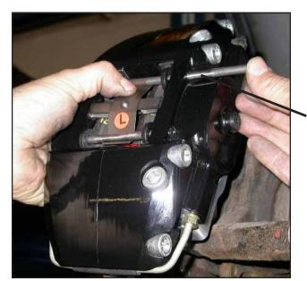
Slide the upper pad-retaining pin into the groove at the top end of the spring clip, and push it through to the inboard side of the caliper.
