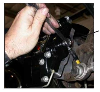
Tighten the banjo bolt to **approximately 14 lbft**, using a 14mm wrench or socket.
