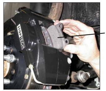
Slide the brake pads into position in the calipers, taking care to ensure that the friction side of each pad is facing the rotor.
