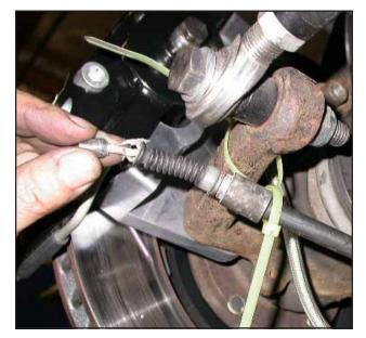
Ensure that the end of the parking brake cable is held securely in place, and that it is not interfering with the movement of any other component. Complete the installation on both sides of the vehicle before bleeding the system.
