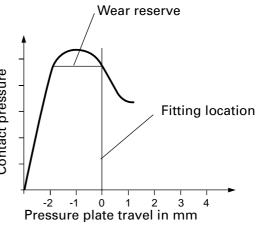
If the position of the main diaphragm spring remains constant over the entire wear range, the associated forces will also remain
