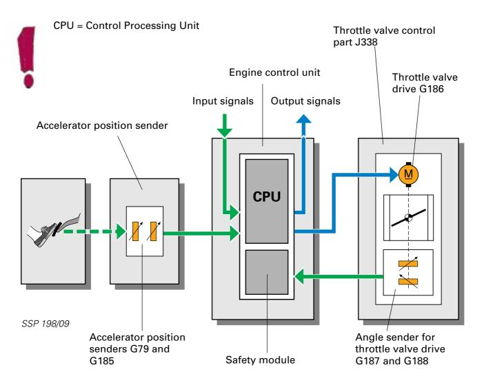
The electronic accelerator controls the engine output electronically and, over and above intake-air control, offers the advantage that functions such as idling speed control, cruise control or engine governing can be executed easily and comfortably. The electronic accelerator is used for reducing and increasing torque and does not adversely affect exhaust emissions.
