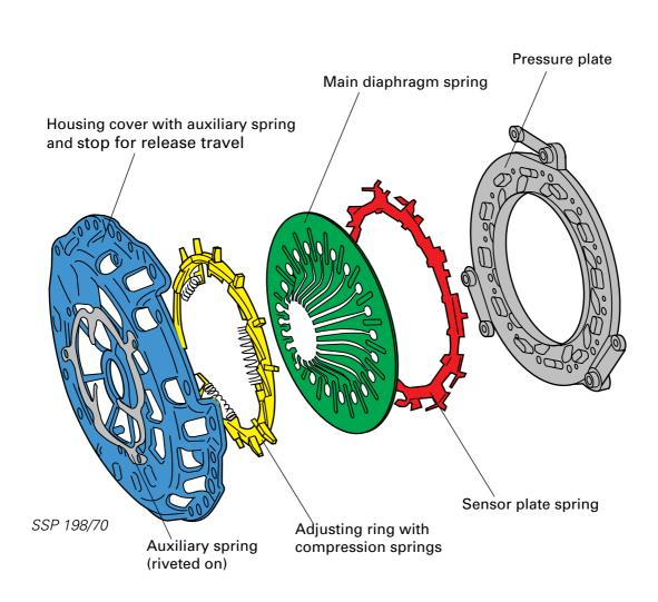
Unlike conventional pressure plates, the main diaphragm spring mounting of the SAC clutch is non-rigid.
