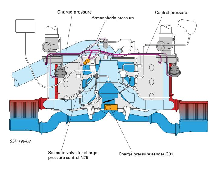
The solenoid valve for charge pressure control N75 changes the opening time to atmospheric pressure according to the signals it receives from the engine control unit (duty cycle).
