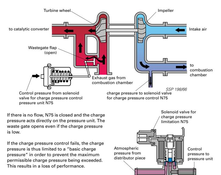
The "basic charge pressure" is the charge pressure (approx. 300 - 400 mbar) which is achieved without regulation (mechanical charge pressure).
