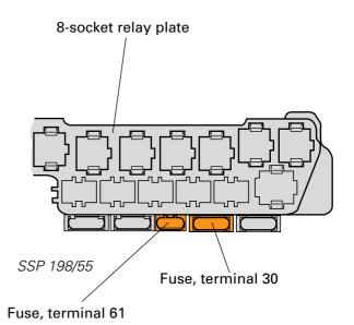
The power supply is protected by a fuse on the 8-socket relay plate. For the correct fuse rating, please refer to wiring diagram. Vehicles equipped with an air
