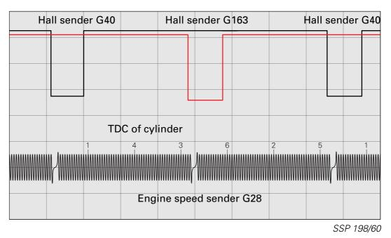
Here, the signals which G40, G163 and G28 generate are shown combined for added clarity. A two-channel oscilloscope does not allow all three signals to be represented. The TDC mark of the belt pulley reflects the TDC of cylinder 3.
