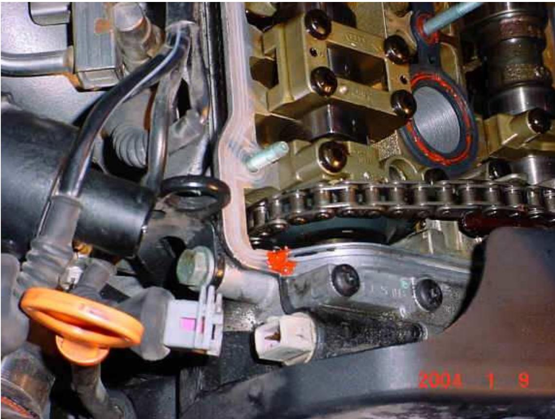
Above you can see the red silicone I used at the ends of the cylinder head. Where this silicone is applied is where my initial leak was. After removing the gasket I noticed that I had been leaking oil around the "valley" as well. In the picture above you can also see the small bead of silicone around the center gasket.
