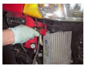
Remove radiator support screw from side of fenders below turn signals.
