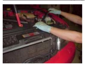
Remove front weather stripping from engine bay.
