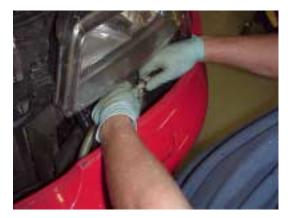
Un-hook by removing black retaining clip.
