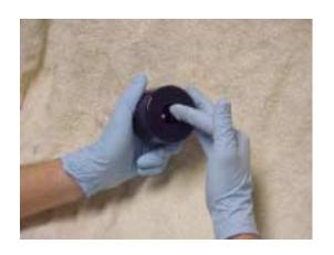
Apply a silicone o-ring lubricant or suitable substitute to the spindle and mount to ease installation of the new mount.
