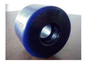
Due to changes in the motor mount housing throughout production of the vehicle the new APR motor mount may need to be shaved slightly to reduce vibration felt in the cockpit.
