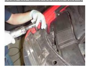
Remove screws in fenders from upper radiator support.
