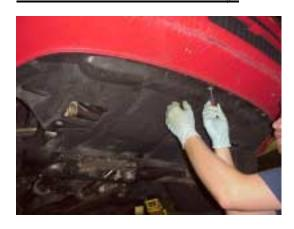
Remove all retaining screws securing the under tray; 10 Total
