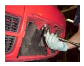
**STEP 6: Remove Inner Fender Well Screws.**
