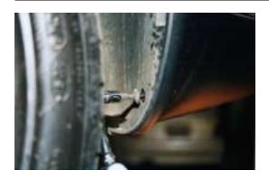
Remove inner fender well screw from bumper located in wheel well.
