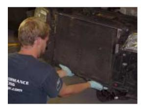
Pull radiator support forward enough to access existing front motor mount.
