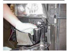
Unbolt bumper shocks, leaving 10mm nuts in place.
