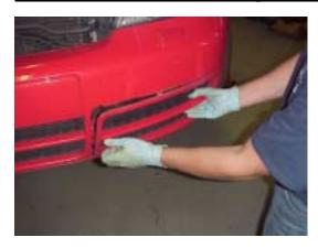
Remove lower bumper inserts next to fog lights by pulling forward firmly but gently at the center.
