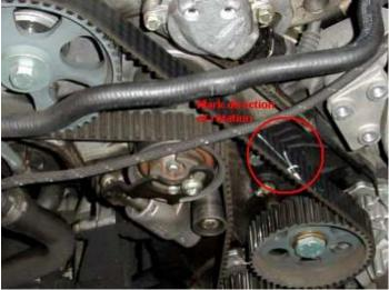
31. Now we reach the moment of no return...time to remove the factory timing belt and (evil) OEM tensioner. Release tension on the belt by loosening the adjustment bolt on the tensioner.
