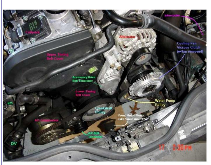
16. Timing Belt (finally): Start by removing the plastic engine cover, to expose the coilpacks. The three fasteners that hold it are loosened by turning them 90 degrees counterclockwise.
