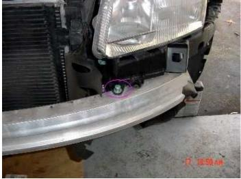
10. Lock Carrier (LC): This part of the body holds the radiator and oil cooler, headlights, horns and some other plumbing, as well as the hood latch. While the LC does not have to be completely removed, it does need to be moved forward several inches to provide the working space needed to change the timing belt. This can be done without draining the radiator, though care must be taken to avoid damaging the various lines that run to it, such as:
