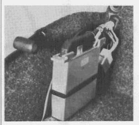
In the Bus, the control unit is located at the right hand side of the engine compartment. The relays are mounted on the left side firewall.
