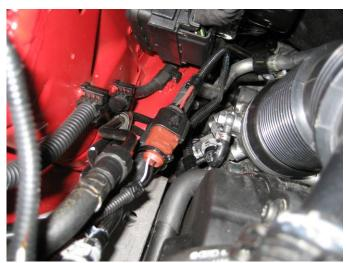
Install supplied hose for the Turbocharger Recirculation from the Recirculation Valve flange, under the A/C service hose, to the Turbocharger Inlet hose. Attach support clip to coolant service line above alternator. Install spring clamps at both ends of the hose.
