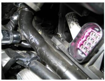
Disconnect electrical connector for Fuel Pressure Sensor G247. This is difficult to see and is below the intake manifold between cylinders 1 and 2.
