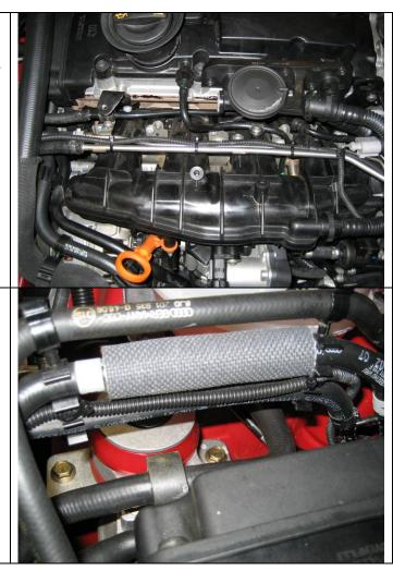
Connect the extension harness to the OEM connector for the Turbocharger Recirculation Valve N249 (near the turbocharger). Zip tie the connector to the A/C pipe on the passenger side of the vehicle, forward of the ABS pump. Place the connector over the rubber buffer on the A/C pipe before you zip tie. Use two zip ties, one at each end of the connector.
