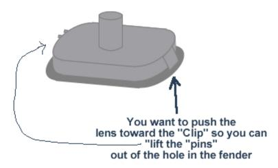
Easiest way I found was to push the lens left and then to the right (with one screw driver)
