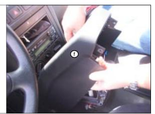
STEP 35. Replace screws (2) ⓓ and screw covers (2) ⓒ (both sides - not shown). TOOLS: Torx Drive (T-20) ₪
