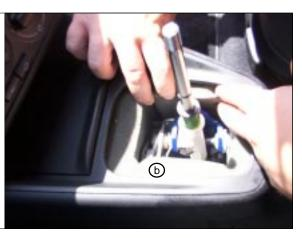
STEP 38. Screw on knob (D). Note: Even knobs that originally "pull off" will screw on.
