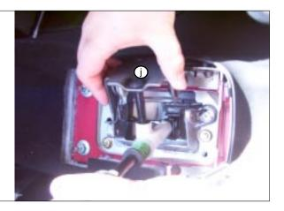
STEP 12. Remove lower cable pin (k). TOOL: Needle Nose Pliers (P)
