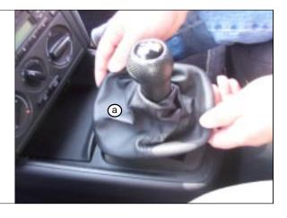
**STEP 40.** Again, test movement of shifter into all gears. DO NOT operate vehicle until all gears can be smoothly and fully engaged.
