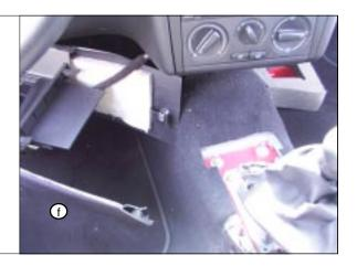
STEP 8. Remove neutral adjustment screw (). TOOL: Wrench (13mm) ()
