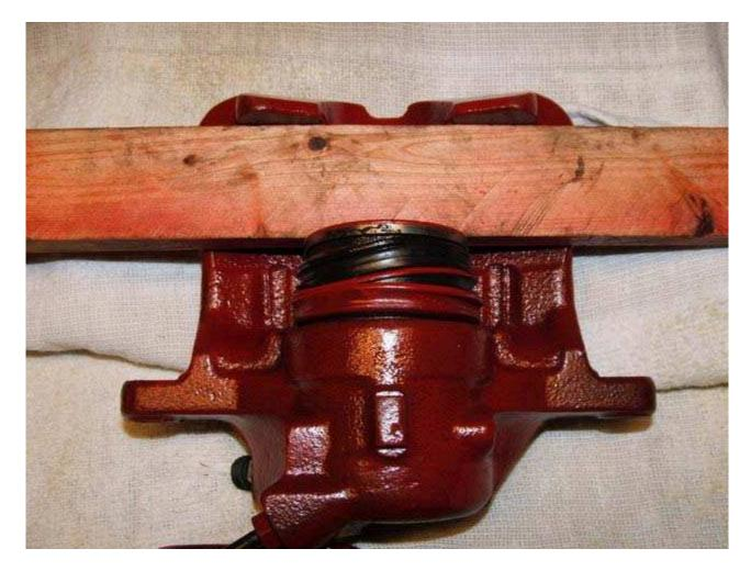
I was carefull with poping out the piston. 40psi worked for me. Use a bunch of brake clean in and out.
