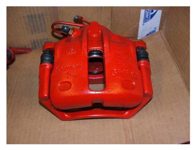
make sure the bleeder screw is facing up when installed to make sure you didnt install them upside down
