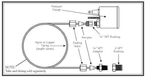
**Diagram C**Proper hookup of the tubing from the gauge to the engine
