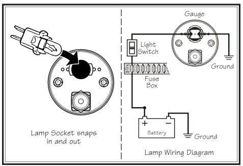
**Diagram A**Proper installation and wiring of lamp socket on all gauges
