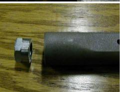
Install the prepared nut in the end of the steering tube.
