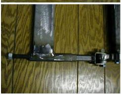
Weld one of the 1/2" by 20 nuts to the end of the 4" by 1/2"by 20 rod for adjusting wheel tension.
