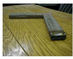
Weld the 8" tube, and the 13" tube together at 90 degrees with the holes in the bar to the inside if the L. Set it with a square, and clamp tightly so there is no twist when welding.
