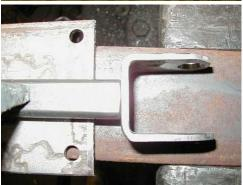
Weld the solid steering shaft to the yoke, centered under the bolt hole, with the flat of the shaft parallel with the bolt. The shaft has to be square with the bolt.
