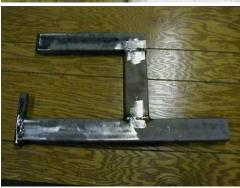
After you have welded the two parts of the frame together. You can remove the the upper bearing, and lower yoke assembly. You should now have a basic frame that looks like this. Installation of the washers in the yoke will allow you to disassemble the unit to this point.
