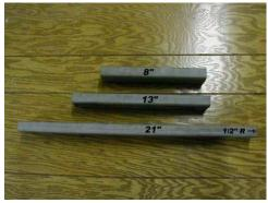
We start with 3 pieces of 1" by 2" tubing at the lengths listed. Other sizes can be used, adjust the lengths accordingly. The longest piece has a 1/2" radius cut on the narrow sides of one end.
