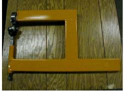
Now go wheel something! This wheel should handle up to 18 ga. steel no problem. Make sure your part is clean, with no paint, or rust on it before wheeling. Wipe parts ever time before wheeling. You can use this wheel with a shot bag to save time, rough it with the bag, and finish on the wheel.
