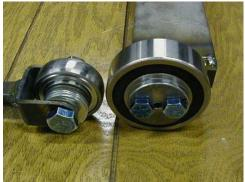
The bottom bearing should have a flat about .075 wide sanded in the center, and blended into the radius. Not totally necessary, but it makes the wheel more effective. Clean and paint as desired.
