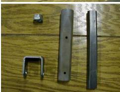
You will need the inner and outer slip joint from a steering shaft, or column, at the lengths listed. Remove the plastic lock so it will slide smoothly. File to fit if necessary.
