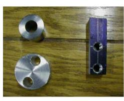
You will need a piece of 1" bar stock the same length as the smaller bearing, with a 1/2" hole drilled through the center.
